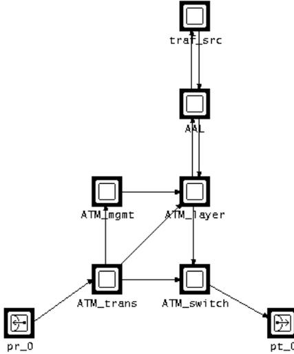
Figure 5: Block Diagram of Source Node in OPNET
