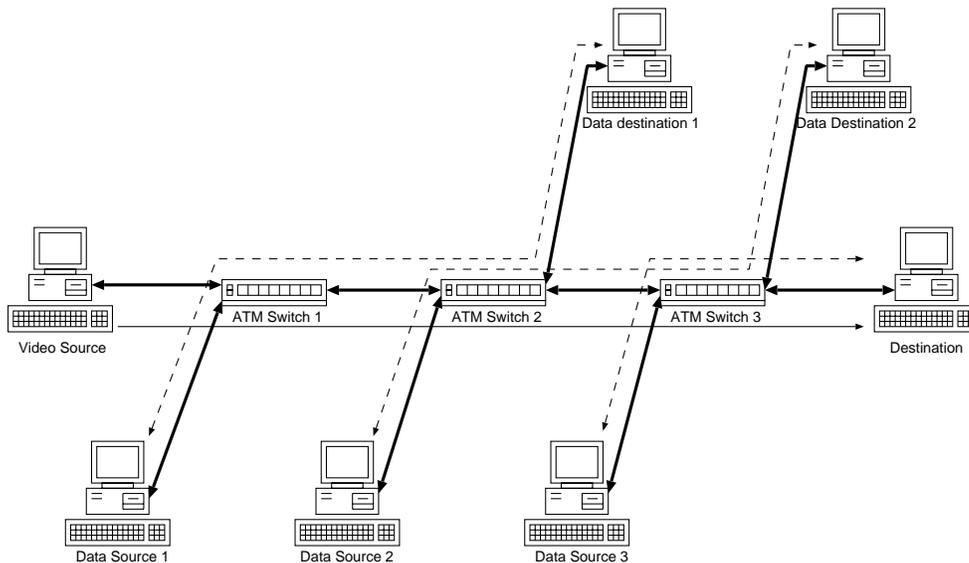
Figure 9: Simulation Model for Multiple Nodes Case
