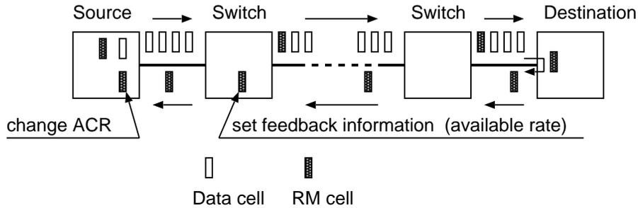
Figure 1: ABR feedback scheme
