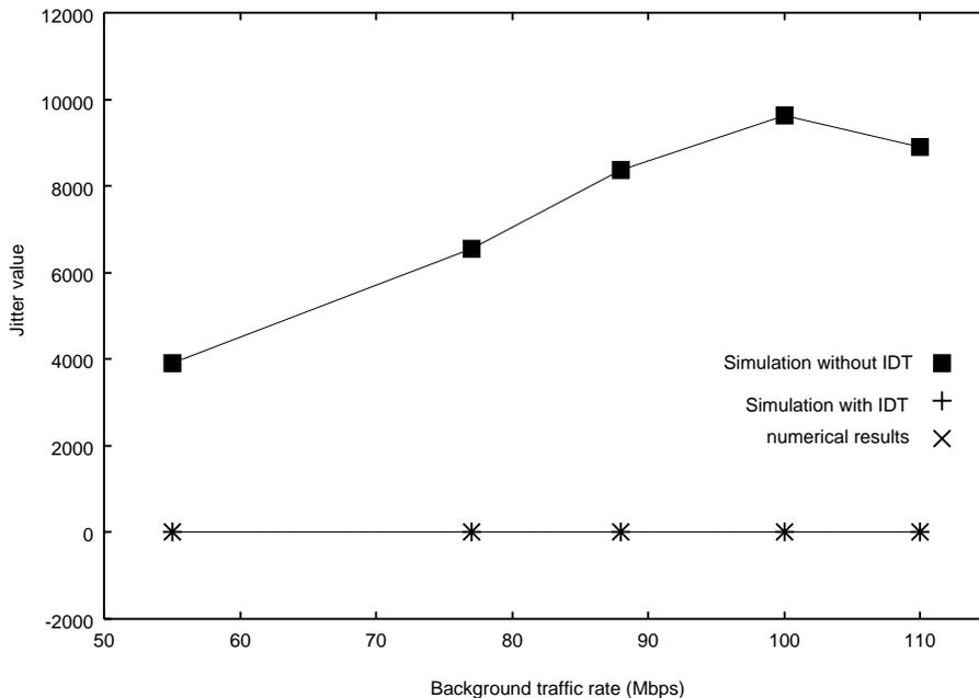
Figure 8: Jitter in Single Node Case
