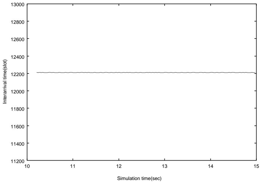
Figure 13: Interarrival Time with IDT in Single Node Case
