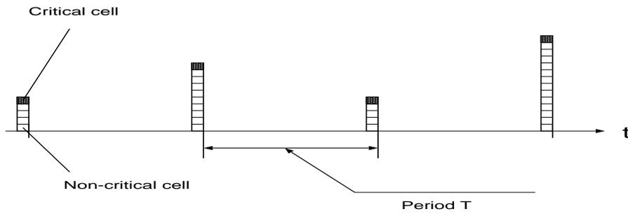
Figure 2: Departure Process at Source Node
