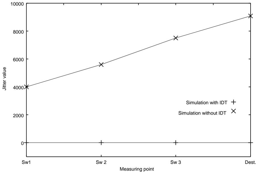
Figure 10: Jitter in Multiple Nodes Case with 50Mbps Background Traffic
