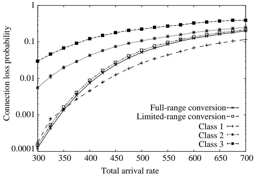
Fig. 12. Connection loss probability vs. total arrival rate for mesh-torus network:  $L = 25$ ,  $W = 32$ ,  $\theta = 9$ , and  $W^{(s)} = 8$ .
