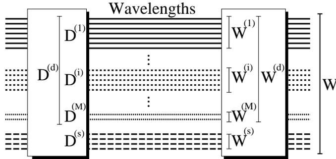
Fig. 1. Shared wavelength allocation method.
