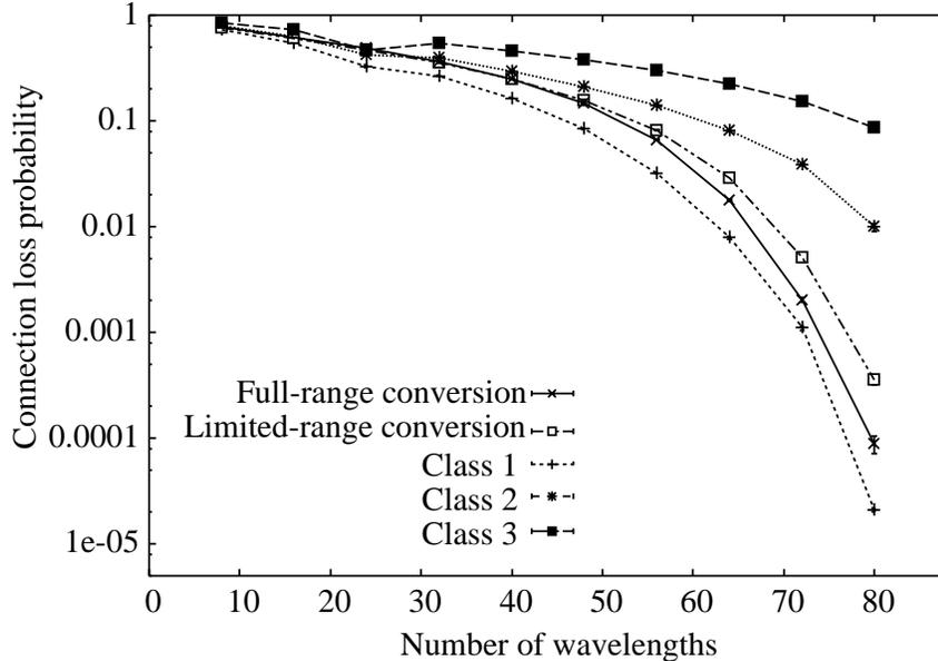
Fig. 10. Connection loss probability vs. the number of wavelengths for ring network:  $L = 10$  and  $\theta = 4$ .
