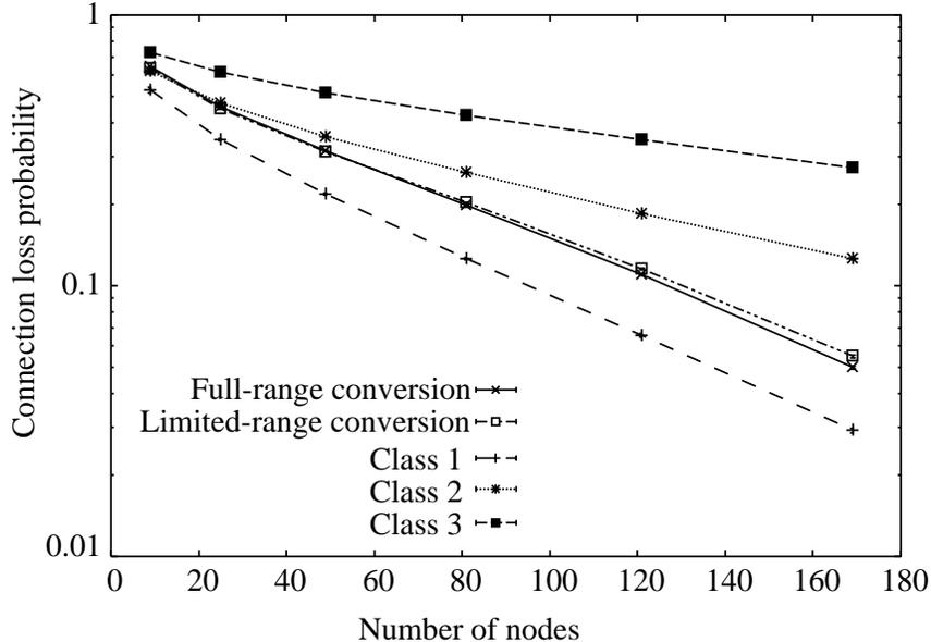
Fig. 13. Connection loss probability vs. number of nodes for mesh-torus network:  $W = 32$ ,  $\theta = 9$ , and  $W^{(s)} = 8$ .
