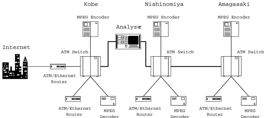
Figure 2: Measuring environment.
