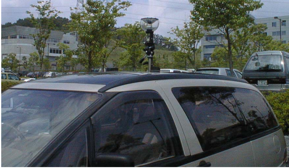
Figure 13: HyperOmni Vision mounted on a car.
