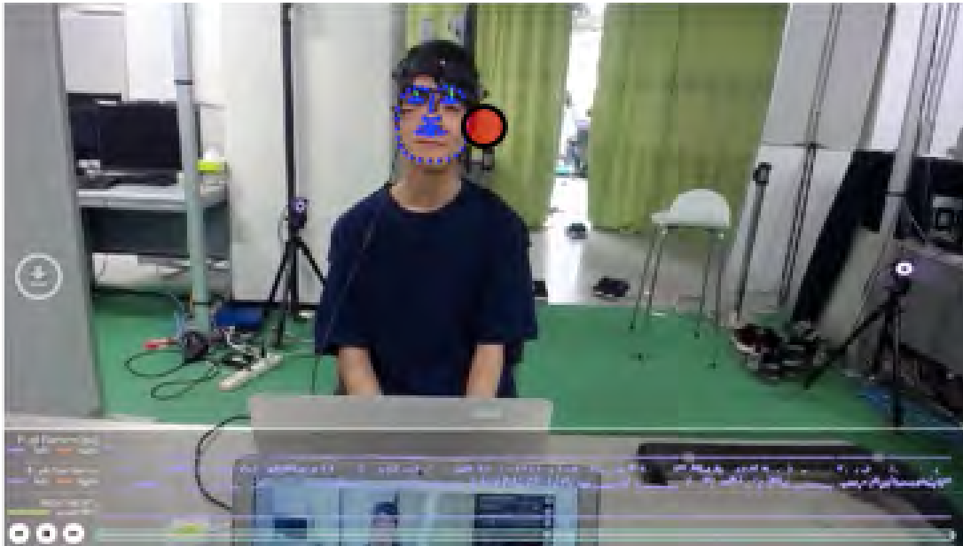
Figure 15. Image obtained from the eye tracker overlaid with a gaze point and the results of facial detection.
