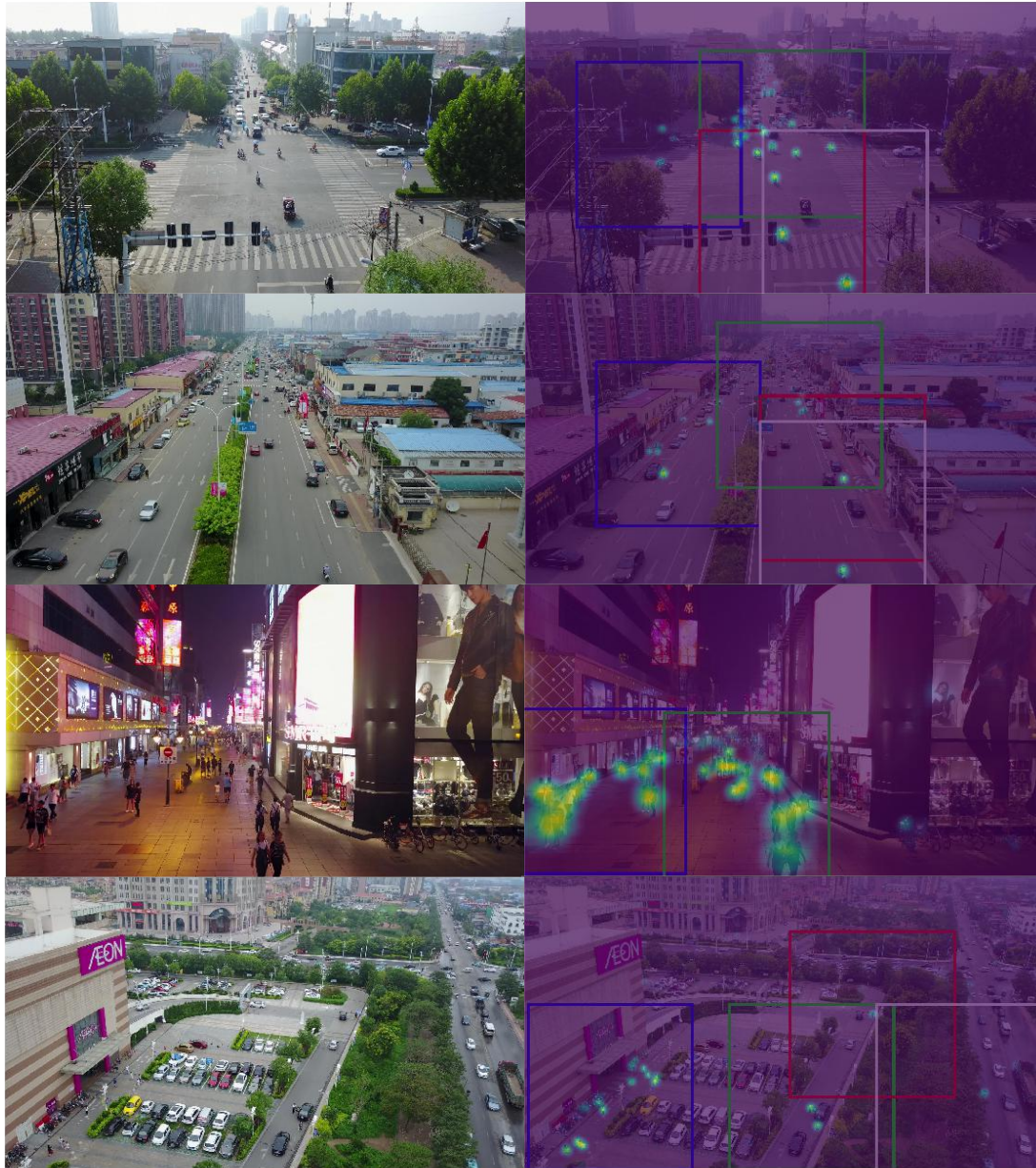
Figure A.17: Visualizations of dense map estimation and patch generation on VisDrone testing dataset (1/3). The size of above aerial images is 1080 \times 1920 and the patch size is 608 \times 608 . Proposal patches are bounded by colorful rectangles.
