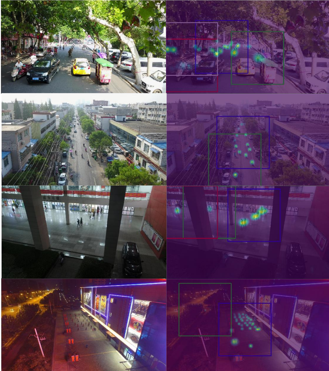
Figure A.18: Visualizations of dense map estimation and patch generation on VisDrone testing dataset (2/3). The size of above aerial images is 1080 \times 1920 and the patch size is 608 \times 608 . Proposal patches are bounded by colorful rectangles.
