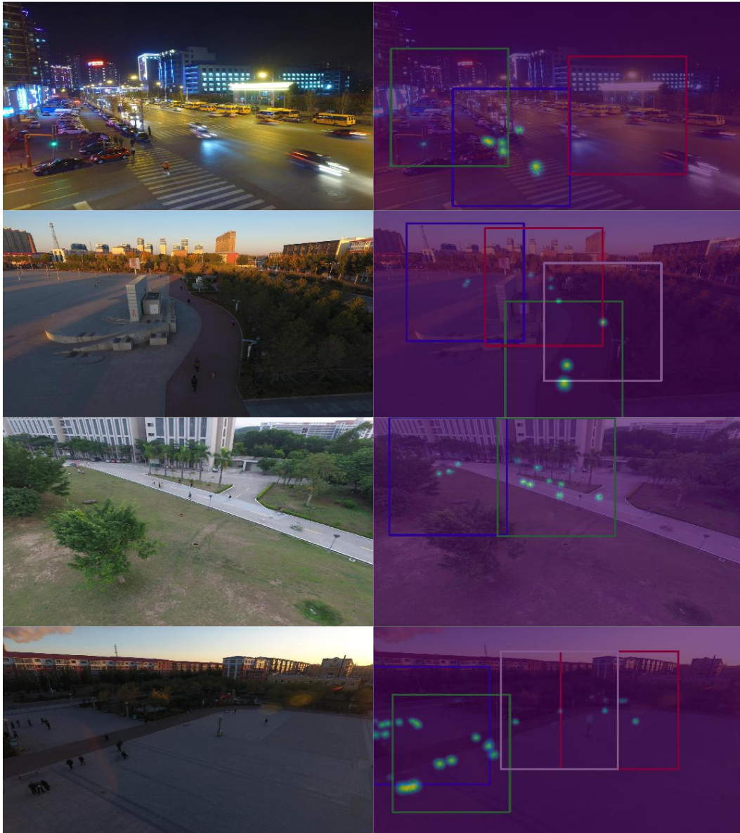
Figure A.19: Visualizations of dense map estimation and patch generation on VisDrone testing dataset (3/3). The size of above aerial images is 1080 \times 1920 and the patch size is 608 \times 608 . Proposal patches are bounded by colorful rectangles.
