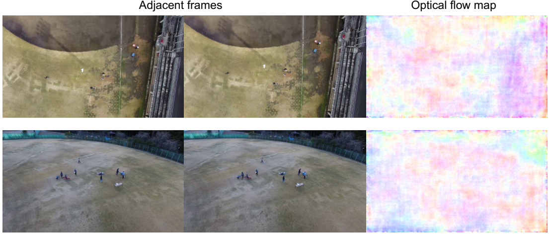
Figure A.14: Visualizations of optical flow maps generated by PWC-Net [5], using Okutama-action Dataset. Due to the tiny size of actor and the drone camera movement, it is challenging to obtain actor motion information from the optical flow.
