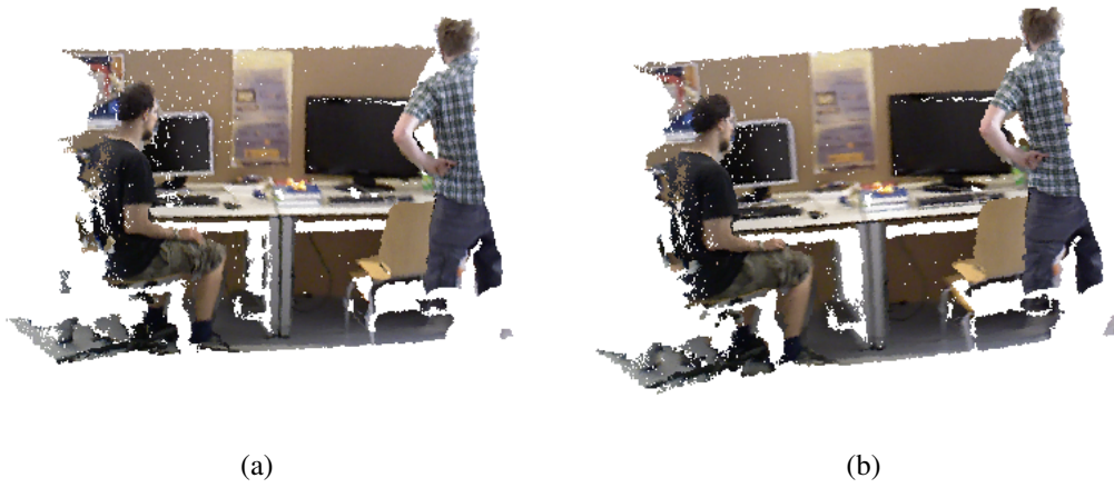
Figure 3.4.: Point cloud representation of two RGB-D frames captured by the Kinect. The SE(3) motion between them can be estimated by using the overlapped points.
