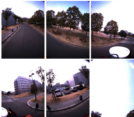
Figure 1 A sampled frame of an acquired omnidirectional video. Right bottom is an image of vertical element camera. Others are horizontal ones.
