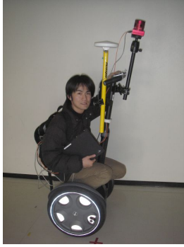
Figure 5 Omnidirectional multi-camera system and GPS receiver.
