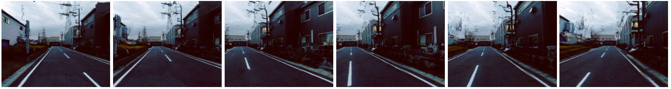
Fig. 1. Example of generated images for virtual camera path that simulates lane change. These images were generated by data captured from the vehicle running on the left lane.
