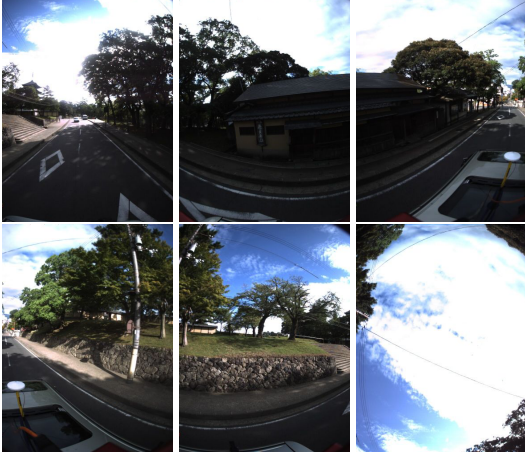
Figure 3. A sampled frame of an acquired omnidirectional video. Right bottom is an image of vertical element camera. Others are horizontal ones.
