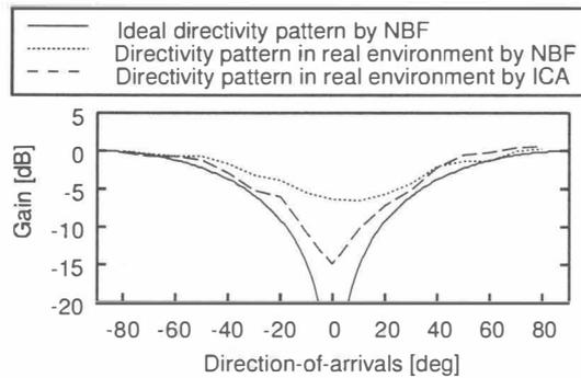
Fig. 5. Directivity patterns shaped by NBF and ICA in ideal environment and real environment which contains element error and reverberation.
