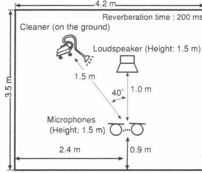
Fig. 4. Layout of reverberant room used in our experiment.
