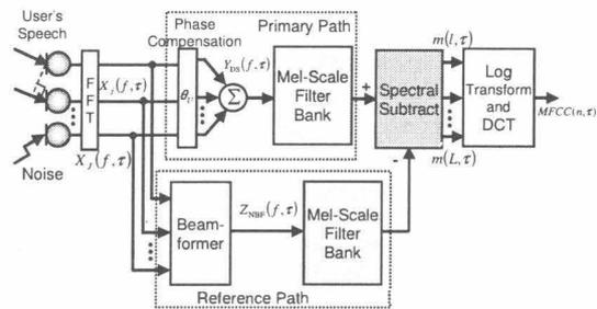
Fig. 1. Block diagram of conventional SSA.
