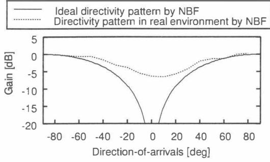
Fig. 2. Directivity patterns shaped by NBF in ideal environment and real environment which contains element error and reverberation.
