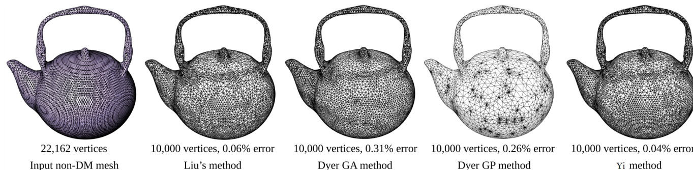
Figure 9. Results from recent methods of mesh simplification. Note that the method of Yi et al. [104] is better in Hausdorff distance (in terms of minimal error) than other methods, such as the methods of Liu et al. [105] and Dyer et al. [87], in geometry-altering (GA) and geometry-preserving (GP) mode even though there is no significant improvement in the visual results. These results are taken from Yi et al. [104].
