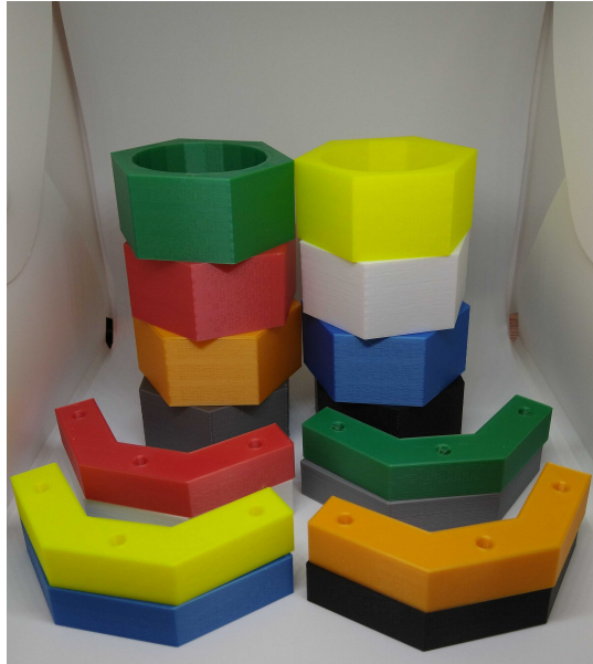
Fig. 16: Objects used for color robustness evaluation. Each object was printed with a PLA filament, 0.2mm layer thickness, and signal amplitude \alpha = 40\% .
