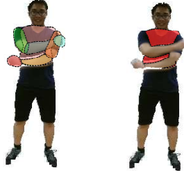
Fig. 5: Left: checking for occlusions by projecting different body part volumes onto a texture. Right: unoccluded regions for the chest body part.
