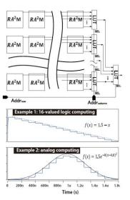
chitecture, which carries out arbitrary hexadecimal functions. Several examples are also given in this figure. By using this technology, the number of devices are reduced to about 30% of traditional **FPGAs** with the same pre-
