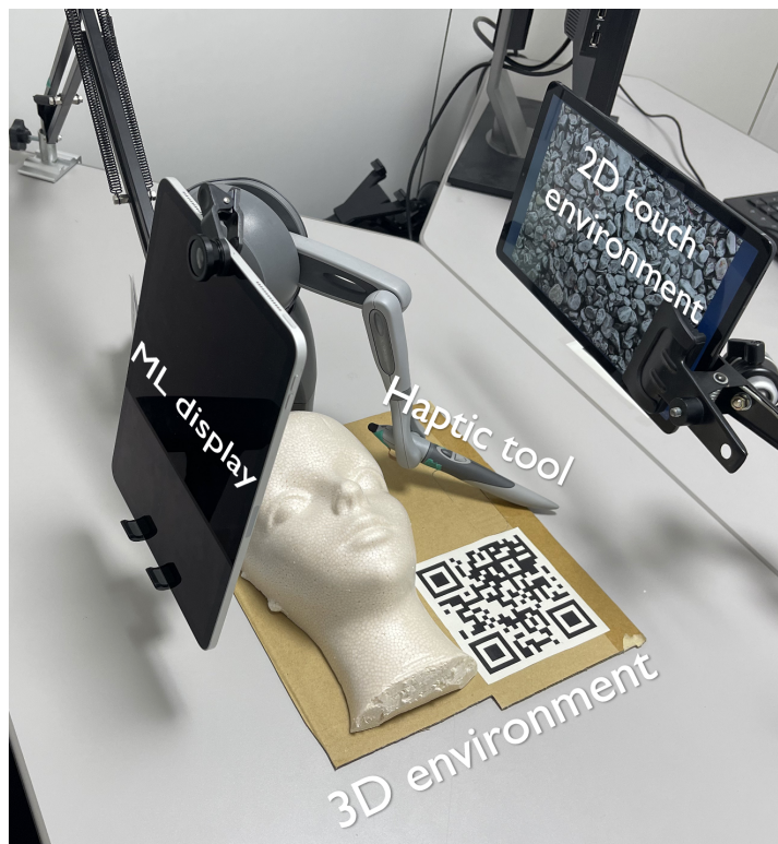
Figure 3.6: Experimental setup showing environments for both experiments. In Exp. 1 , a touch tablet (labeled ‘2D touch environment’) was used for haptic interactions. In Exp. 2 , the touch tablet was swapped out for a foam human mannequin head (labeled ‘3D environment’).
