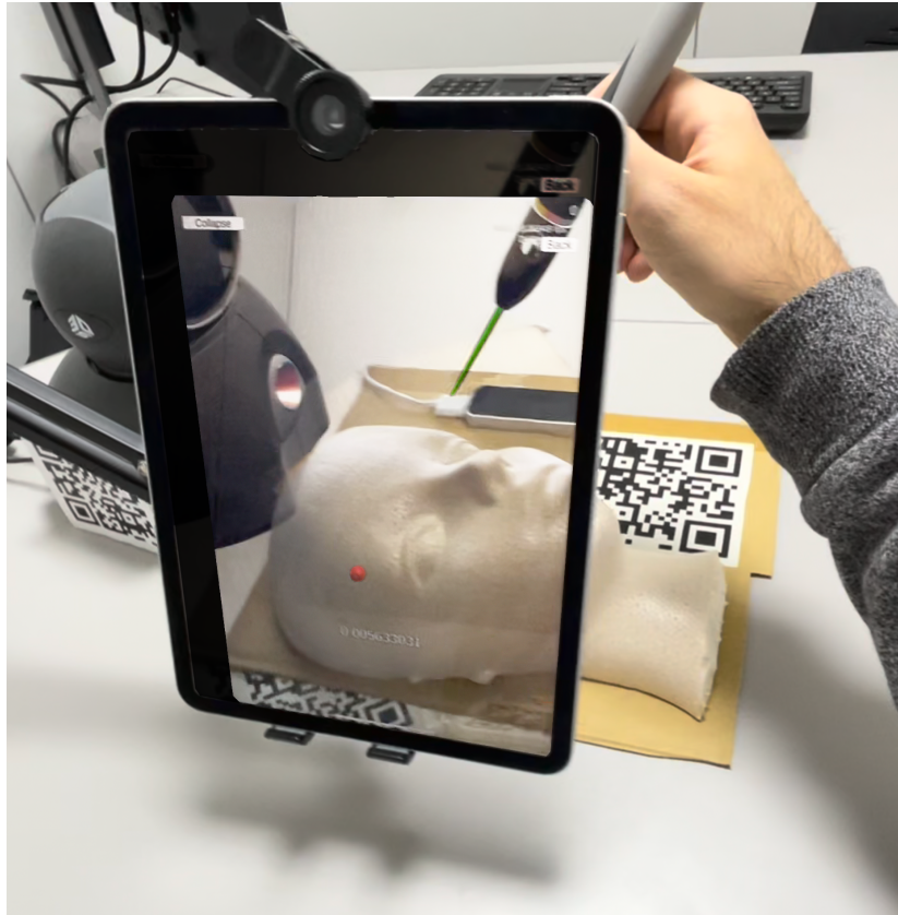
Figure 3.10: Setup for needle injection experiment (Exp. 2). A foam mannequin head is semi-transparently rendered on the ML display while a user is moving a tool equipped with a virtual needle (green). In the configuration shown here, UP rendering is enabled and a red spherical touch target is presented inside the mannequin head.
