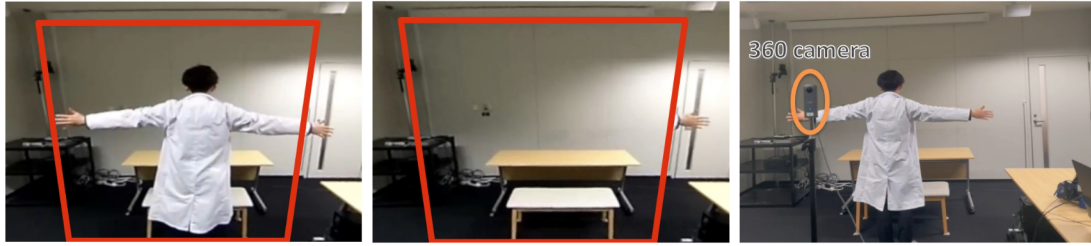
Figure 4.1: The user body is visible in a 360 panorama image before filling a certain area which was surrounded by red line (left). On the other hand, the user body is invisible in the certain area after filling this area (center) while the user is in this area in the real environment (right).
