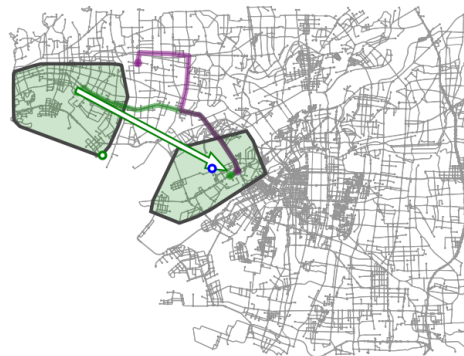
Figure 5.8: Dest. Subroute Conn.: Find and connect dest. subroute (green line) to basis route (purple line)
