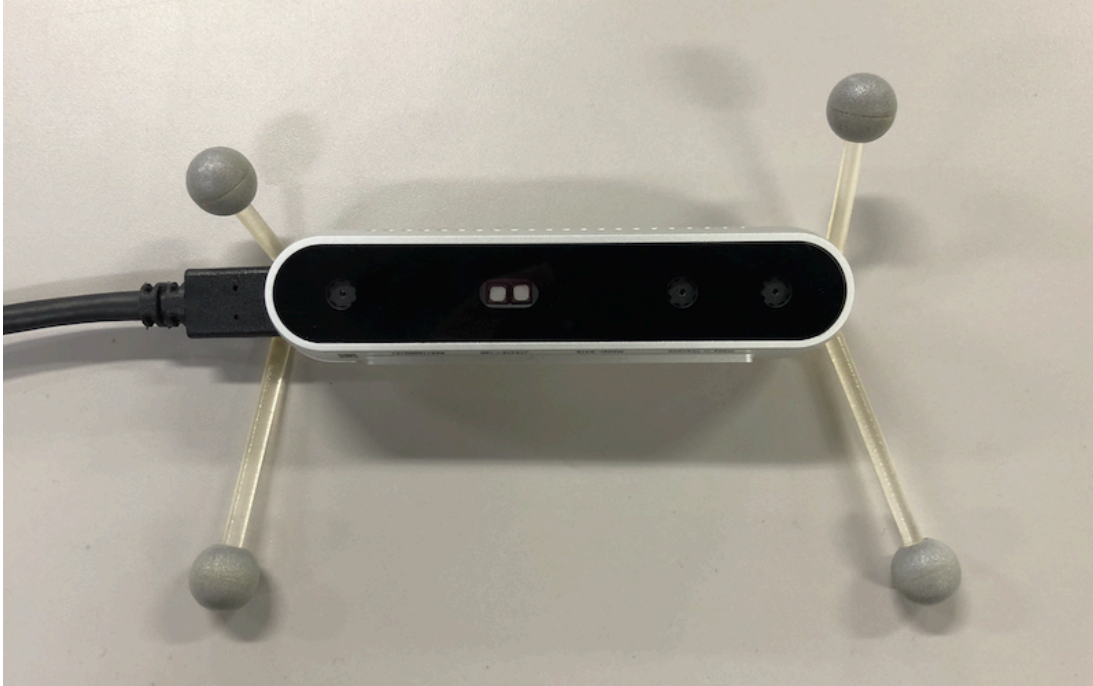
Figure 43: The depth camera with retro-reflective markers. The markers are arranged to register marker set as the origin of the camera coordinate system.
