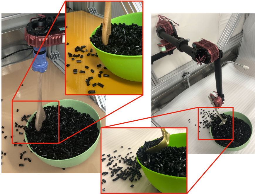
Figure 3.2. This figure provides examples of contact-rich kitchen tasks, where unsafe and intensive contact behaviors can result in damage to the robot or its environment.
