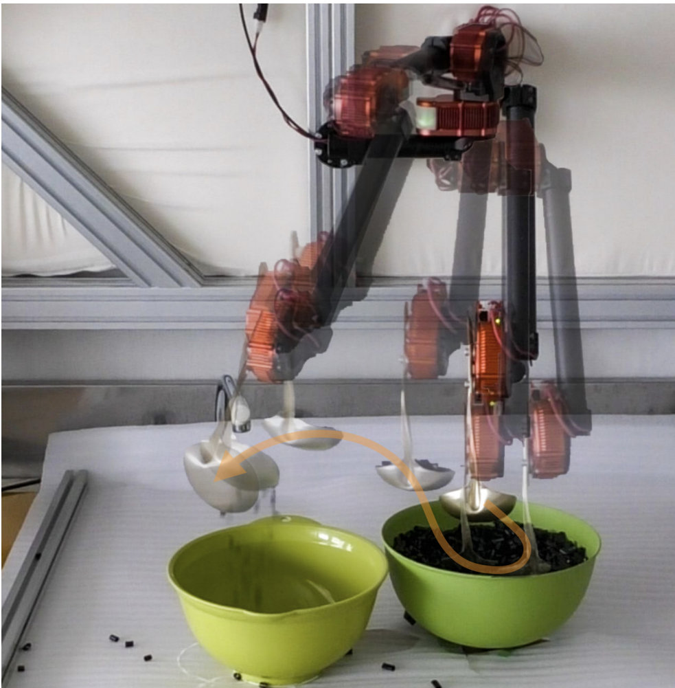
Figure 3.13. This figure illustrates the scooping task trajectory. The orange line showcases the scooping trajectory from the front view.
