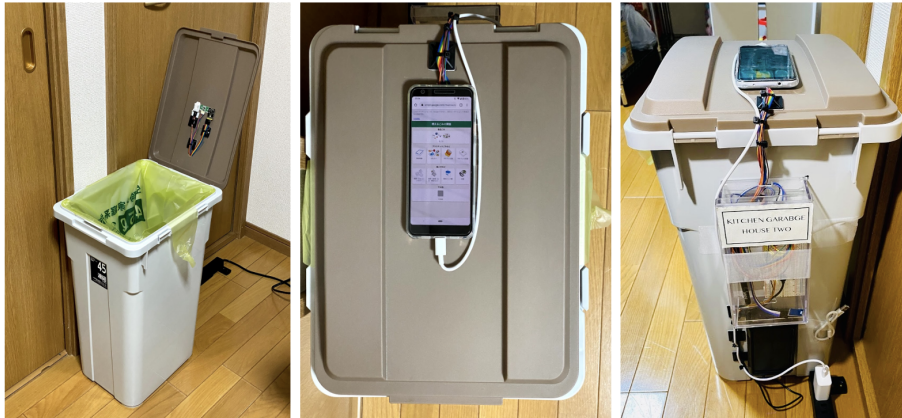
Figure 4.3: Smart garbage bin system deployed in a household
