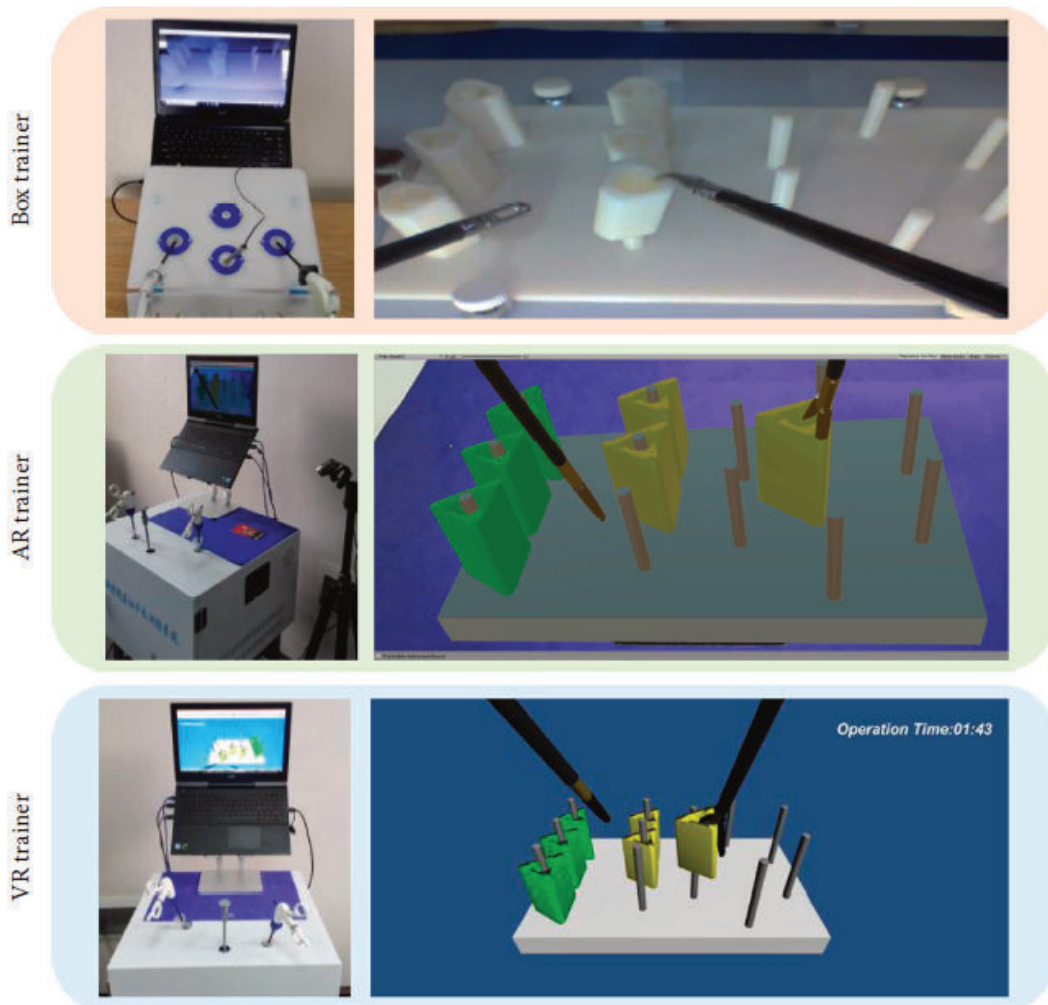
Figure 2.6: Peg transfer simulator on box, AR, and VR platforms [176].
