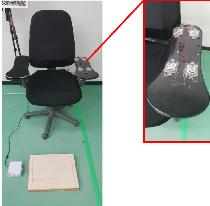
Figure 4.10: Chair Force Sensors developed
