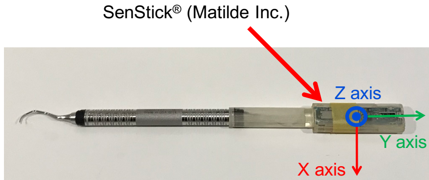
Figure 2.3. Hand scaler equipped with an IMU sensor
