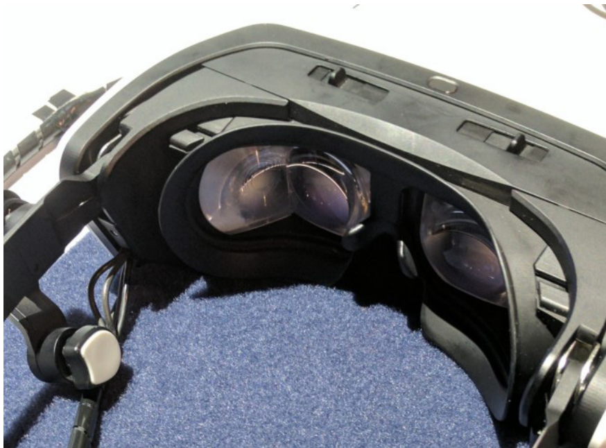
Figure 2.22: Panasonic HMD uses two fused lenses.
