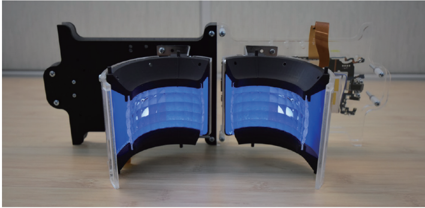
Figure 2.23: HMD with microlensarray for wide horizontal FoV [89].
