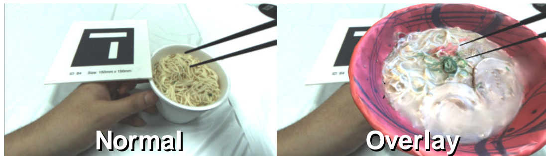
Figure 3.1: Left) Somen noodles in a cup with an AR marker ( Normal condition in the experiment). Right) Overlaid 3D model of ramen noodles ( Overlay condition in the experiment). Although realistic, the model appearance does not change in accordance with the deformation of the actual food. It also causes an occlusion problem.
