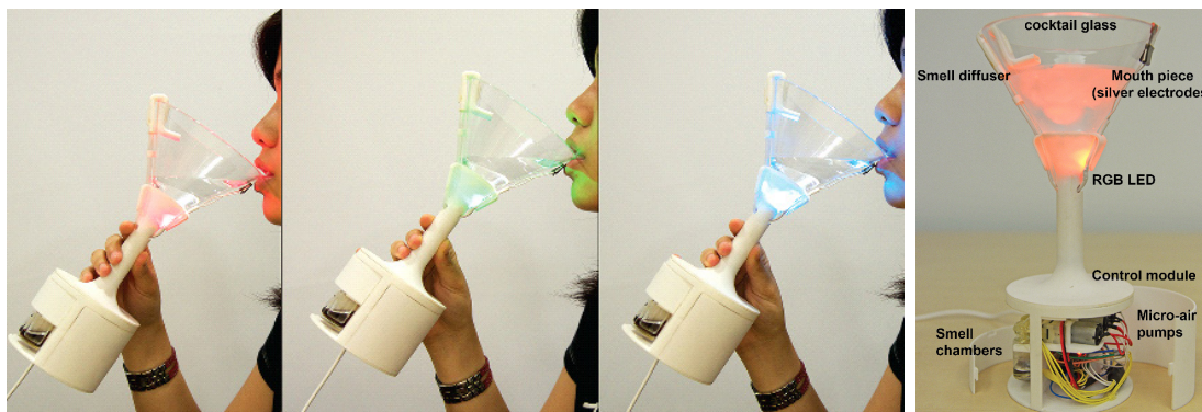
Figure 2.5: Gustatory manipulation interface that changes taste by multisensory presentation with LED coloring, olfactory display, and electric taste [10]
