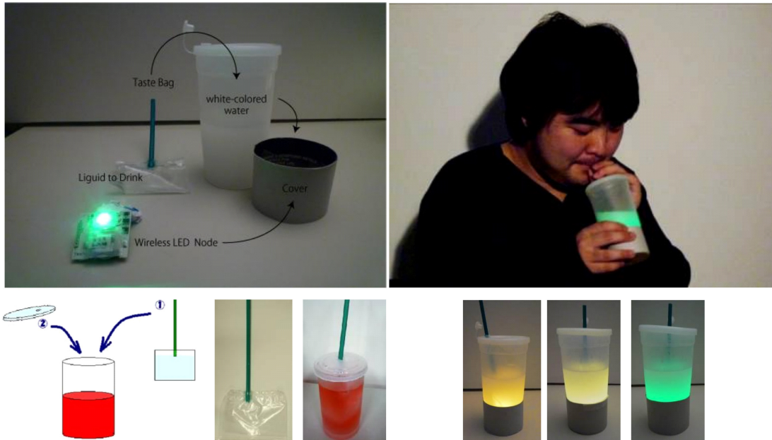
Figure 2.4: A gustatory manipulation interface that changes multisensory flavor perception through LED coloring [9]. Top) overview. Bottom left) Method to separate the colored liquid from the beverage so as not to change the beverage's composition. Bottom right) in operation.
