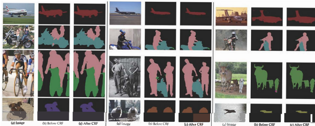
Figure 2.19: DeepLab results before and after input images and Conditional Random Fields (CRFs) when using the PASCAL VOC 2012 dataset [81].
