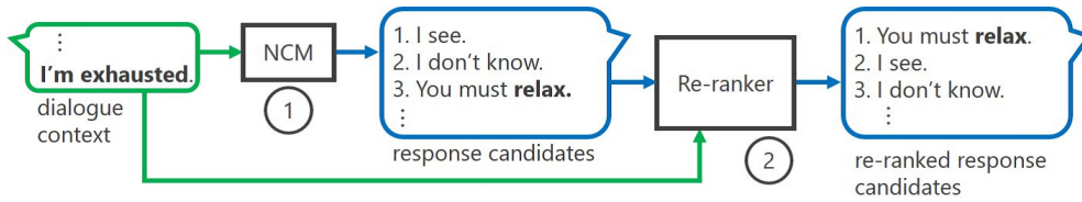
Figure 4.1.: Neural conversational model+re-ranking; Selects the response based on knowledge that I be exhausted and relax have a causality relation.
