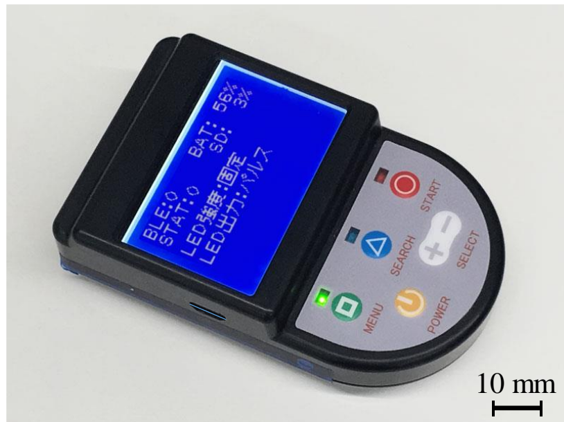
Fig. 1.2 Photograph of the device for lipid concentration detection by detecting the blood scattering properties [28].
