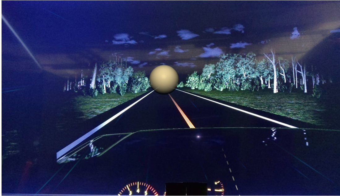
Figure 3.8: The view of the front monitor, featuring the calibration procedure and the blocking of the car speedometer arrow reading from the participant's view.
