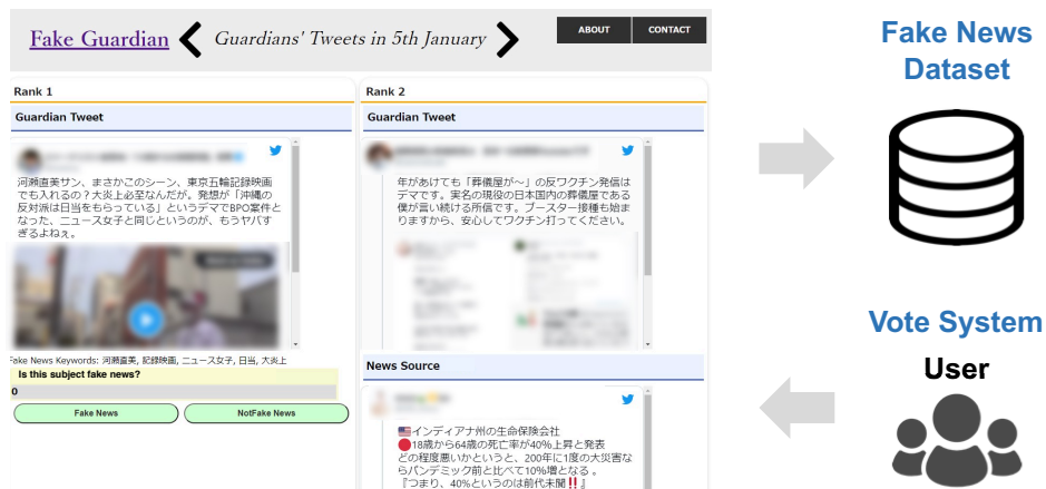
Figure 4.11.: Overview of Fake Guardian: Our system extracts noteworthy guardian tweets against fake news from Twitter on the backend and shows the processed data on the frontend.
