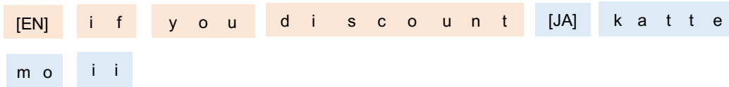
Figure 4.6: Overview of the Direct ASR (TagLID) approach. Given CS speech, it predicts language ID tag like “[EN]” every switching position, followed by the corresponding monolingual character sequences.
