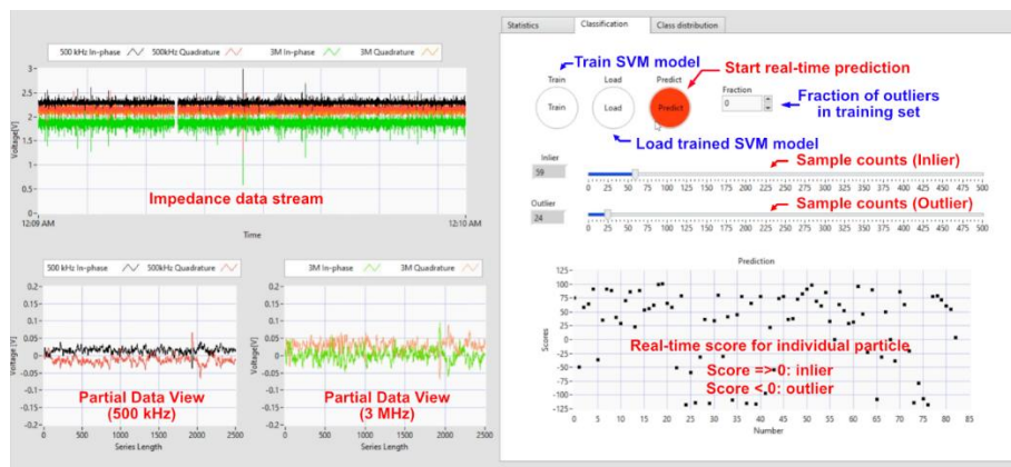
Fig. 3.29: User interface for the online training and prediction of the machine learning algorithm. The one-class SVM model was employed in this work. Users can train the model with reference targets by clicking the “Train” button at any time. The trained model can be loaded into the program by clicking the “Load” button. Clicking the “Predict” button means starting the real-time recognition of individual particles. The trained SVM model
