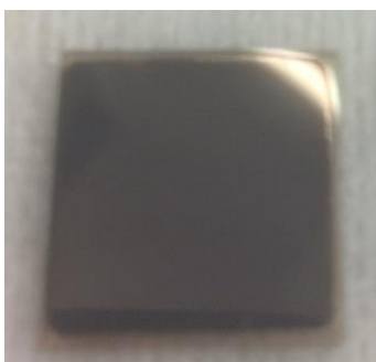
Figure B.4 Photo image of the sputtered film using \text{Cs}_3\text{Bi}_2\text{I}_9 powder.
