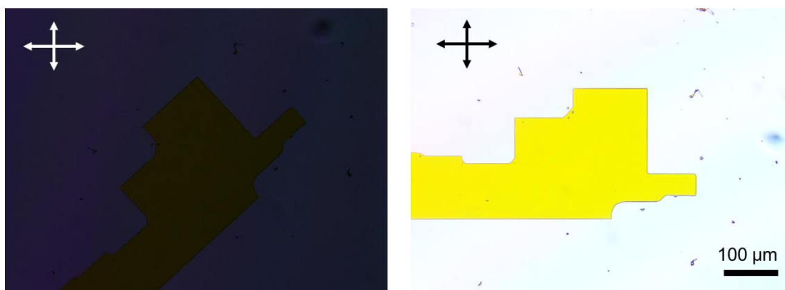
Fig. 2.3.2: Polarized optical micrographs of MAPbBr 3 crystal grown between glass/glass substrates. The horizontal and vertical arrows in the images indicate the polarizer and analyzer directions of the crossed nicols, respectively.
