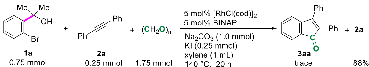
Scheme 4-6. Carbonylative annulation with paraformaldehyde.
