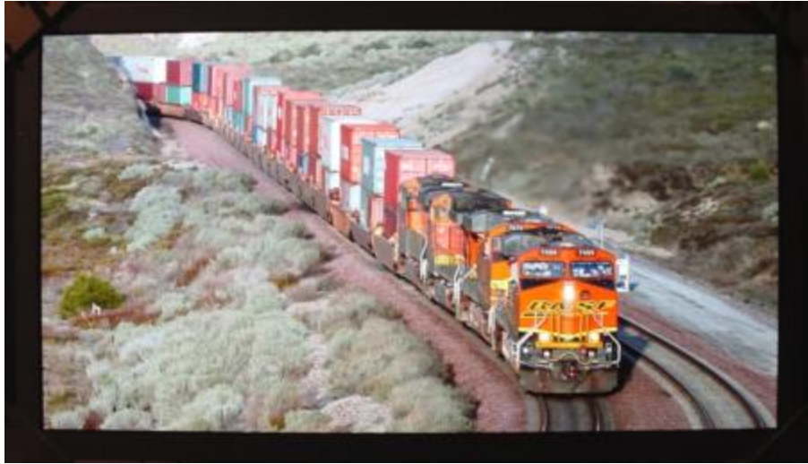
Fig. 83 40-inch diagonal AM-OLED display fabricated in the Gen. 6 line..
