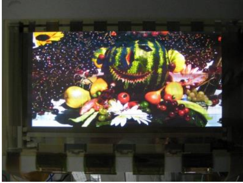
Fig. 66 Scanner-integrated 8-inch diagonal UWXGA AM-OLED display.
