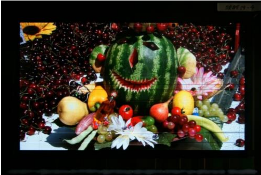
Fig. 77 9.9-inch diagonal qHD AM-OLED display with c-IGO TFT.
