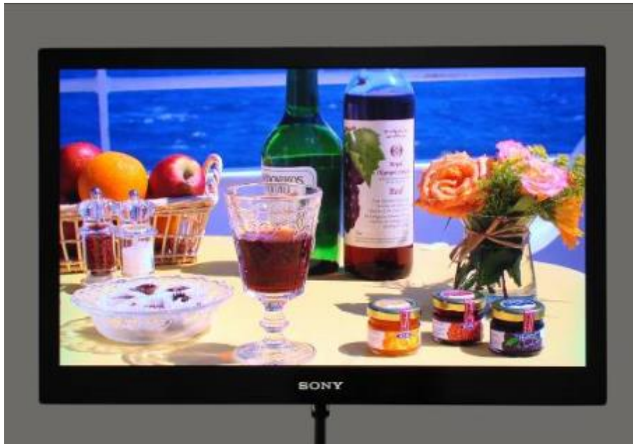
Fig. 42 27.3-inch diagonal FHD \mu\text{c-Si} TFT driven AM-OLED display.
