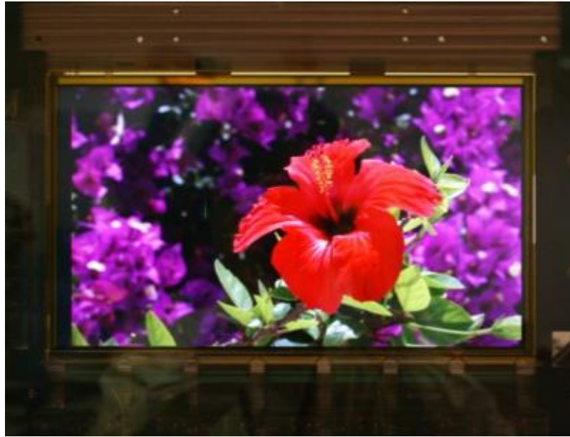
Fig. 58 11.7-inch diagonal qHD a-IGZO TFT driven AM-OLED display.
