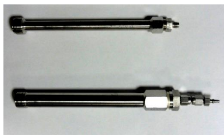
Figure 2-10. Photograph of RC1, top, and RC2, bottom, reactor columns.
