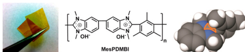
Figure 1-12. A stable hydroxide-conducting polymer. [21b]
