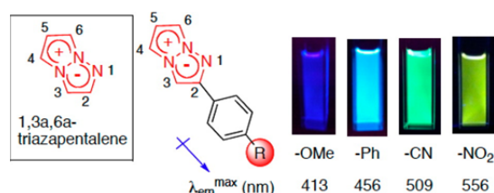
Figure 6-8. Highly fluorescent 2,5-disubstituted-1,3a,6a-triazapentalene. [122]
