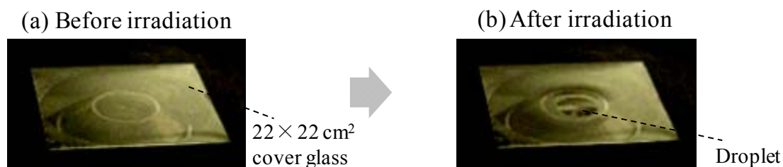
Figure 3.1 Photographs of a sample (a) before and (b) after laser irradiation for 300 sec. The top of an objective lens is clearly identified through the solution and the cover glass in (a), while dense liquid droplet is observed in the center of the glass in (b).
