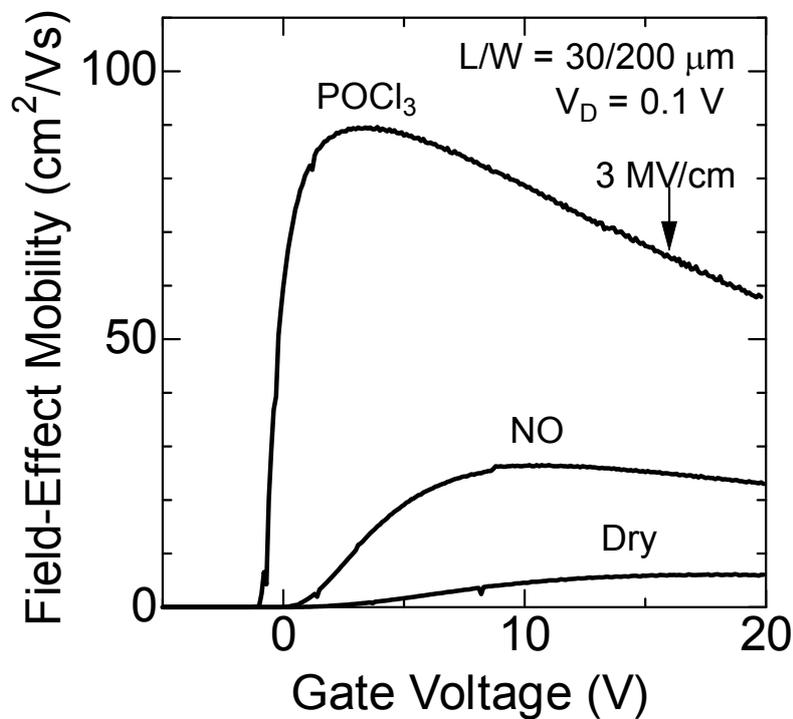
Fig.3.6. Field-effect mobility of 4H-SiC MOSFETs fabricated on the Si-face by dry oxidation, NO annealing, and the  $\text{POCl}_3$  annealing at 1000 °C.
