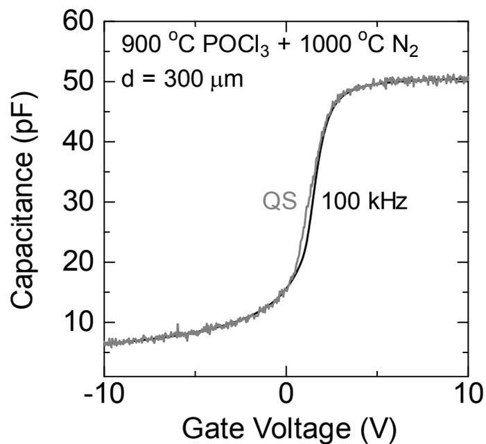
(b) POCl<sub>3</sub> annealing at 900 °C followed by N<sub>2</sub> annealing at 1000 °C (sample D)
