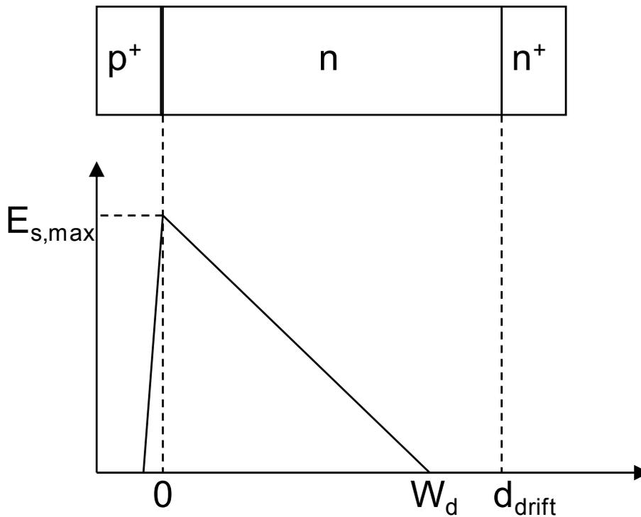
Fig. 1.5. The relationship between the electric field and distance in a drift layer with a one-sided abrupt p<sup>+</sup>-n junction.
