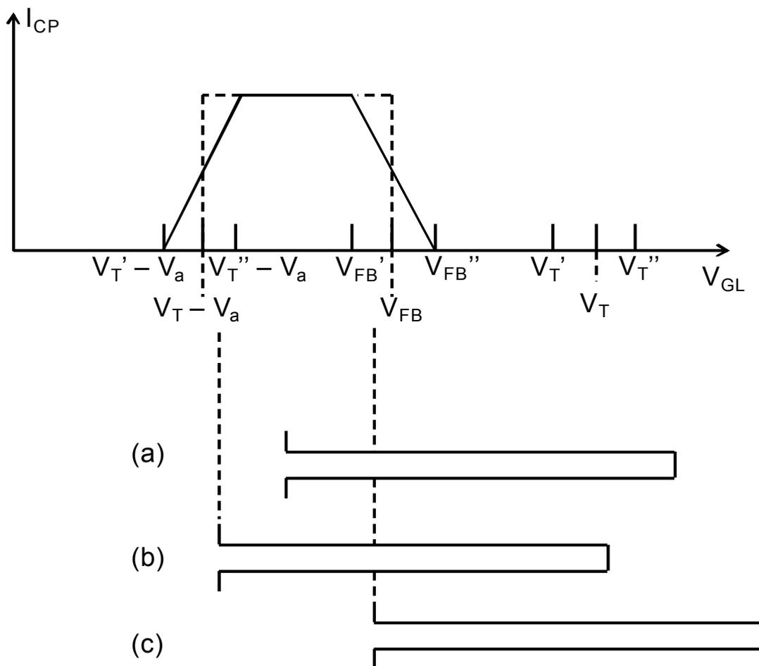
Fig. 5.9. Influence of interface states on charge-pumping curves for n-channel MOSFETs, assuming both donor- and acceptor-like interface states.
