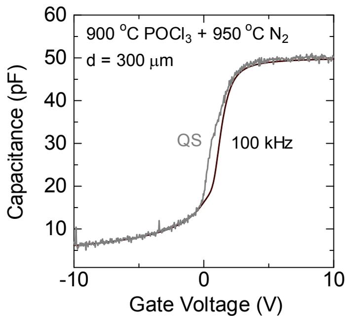
(a) POCl<sub>3</sub> annealing at 900 °C followed by N<sub>2</sub> annealing at 950 °C (sample C)
