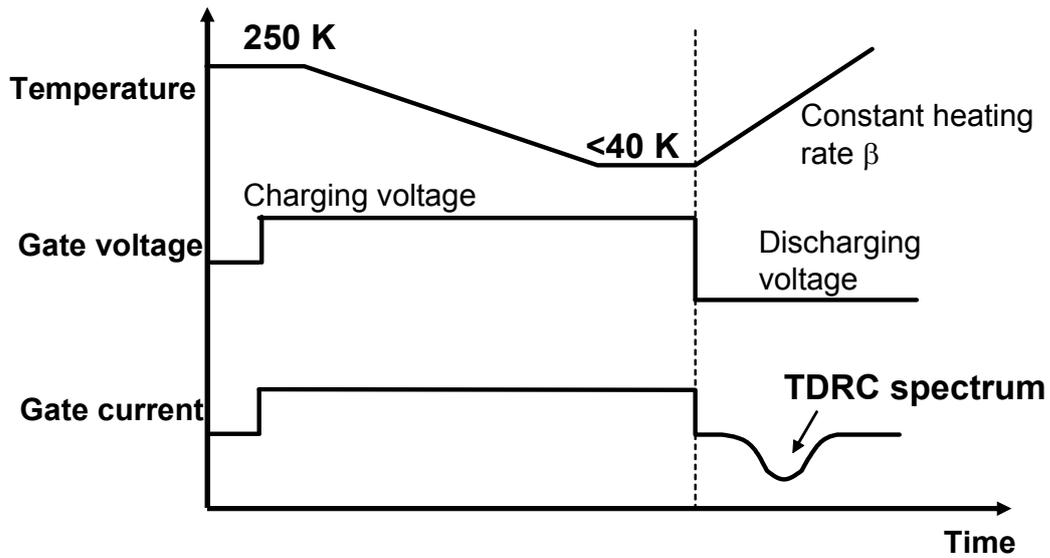
Fig. 4.2. Overview of thermal dielectric relaxation current (TDRC) method.
