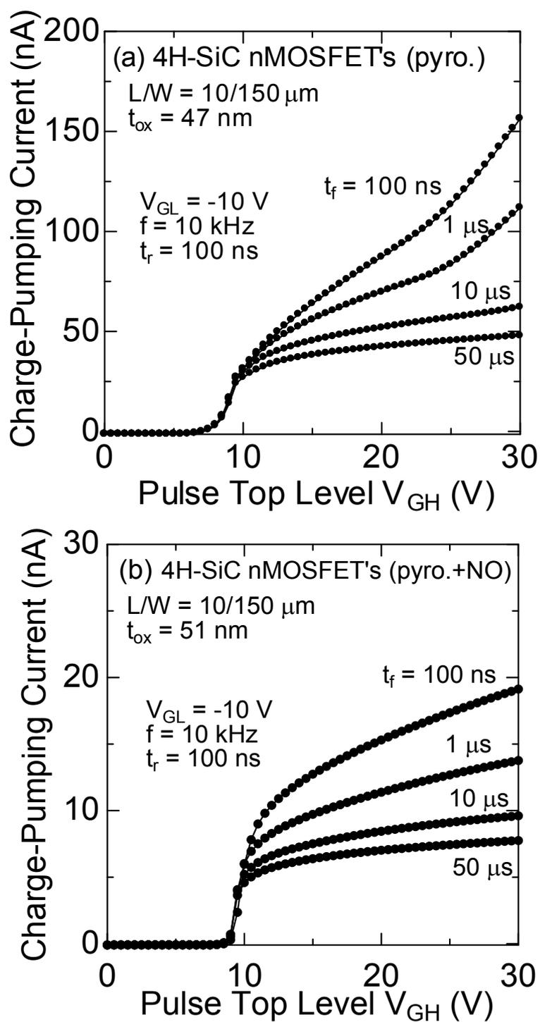
Fig. 5.7. Pulse-fall-time dependence of amplitude-sweep charge-pumping curves for (a) unannealed n-channel 4H-SiC MOSFETs and (b) NO-annealed 4H-SiC n-channel MOSFETs with a gate length  $L = 10 \mu\text{m}$ , and gate width  $W = 150 \mu\text{m}$ . Pulse base level  $V_{\text{GL}}$  is fixed at  $-10 \text{ V}$ . Pulse frequency  $f = 10 \text{ kHz}$ , and pulse rise time  $t_r = 100 \text{ ns}$ .
