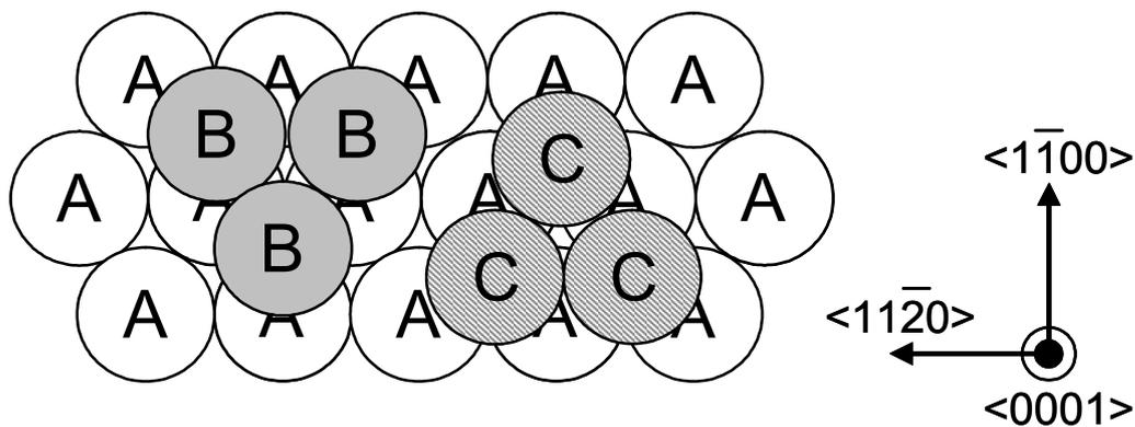
Fig. 1.1. Close-packed structure filled up with many balls. Each Si-C bilayer can be situated in one of three possible positions, which are denoted by A, B, and C.
