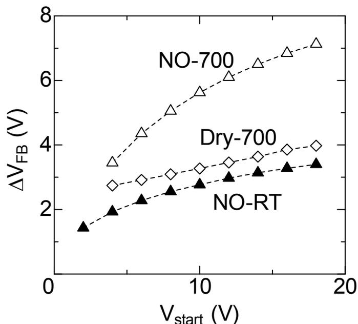
Fig. 6.3. Relationship between start voltage ( $V_{\text{start}}$ ) and flatband voltage shift ( $\Delta V_{\text{FB}}$ ) in high-frequency  $C-V$  measurements for C-face 4H-SiC MOS capacitors fabricated by the Dry-700, NO-700 and NO-RT processes.
