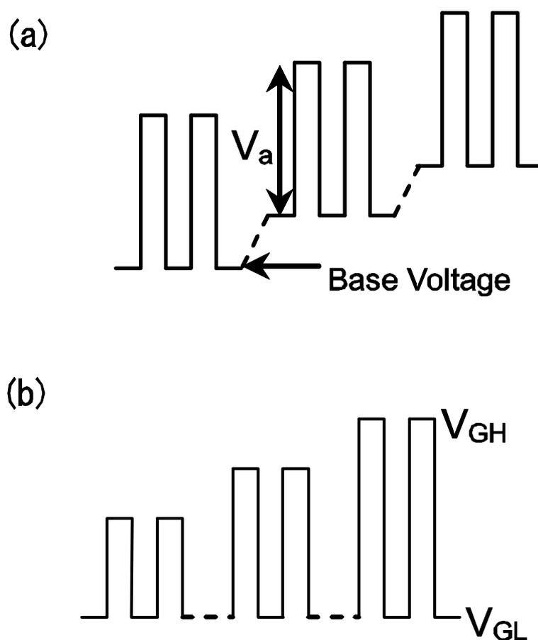
Fig. 5.4. Pulse trains for (a) base-sweep and (b) amplitude-sweep charge-pumping measurements.
