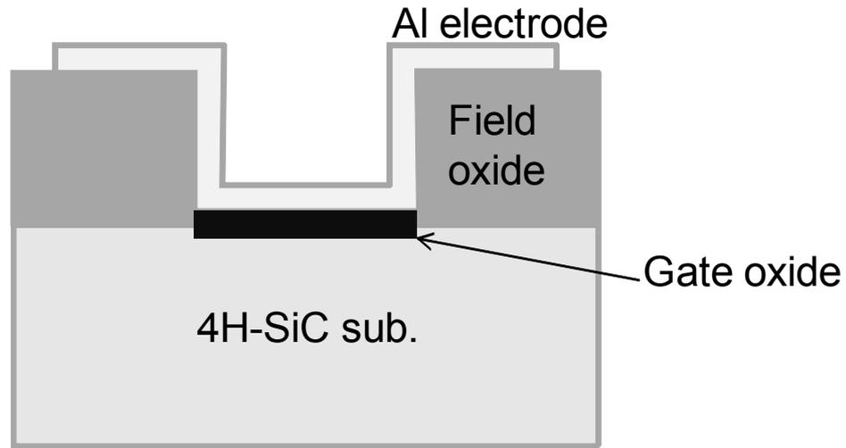
Fig. 3.9. Cross section of a MOS capacitor for the reliability measurements.
