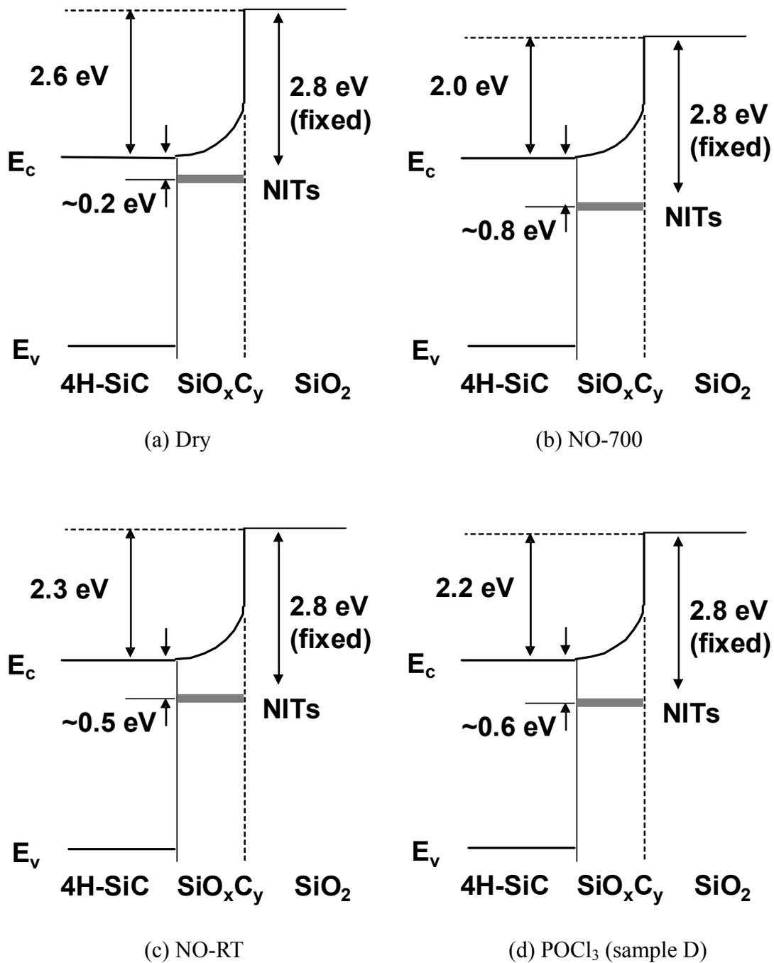
Fig. 6.19. Speculated models of deep NITs for C-face MOS structures. The energy position of NITs changes with the conduction band offset between 4H-SiC and SiO<sub>2</sub> because the energy position of NITs are 2.8 eV below the conduction band edge of SiO<sub>2</sub> [11, 12].
