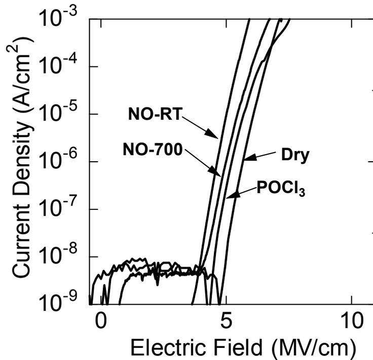
Fig. 6.17.  $J$ – $\mathcal{E}_{\text{ox}}$  characteristics of dry, NO-700, NO-RT, and POCl<sub>3</sub>-anenaled (sample D) MOS capacitors on C-face 4H-SiC.
