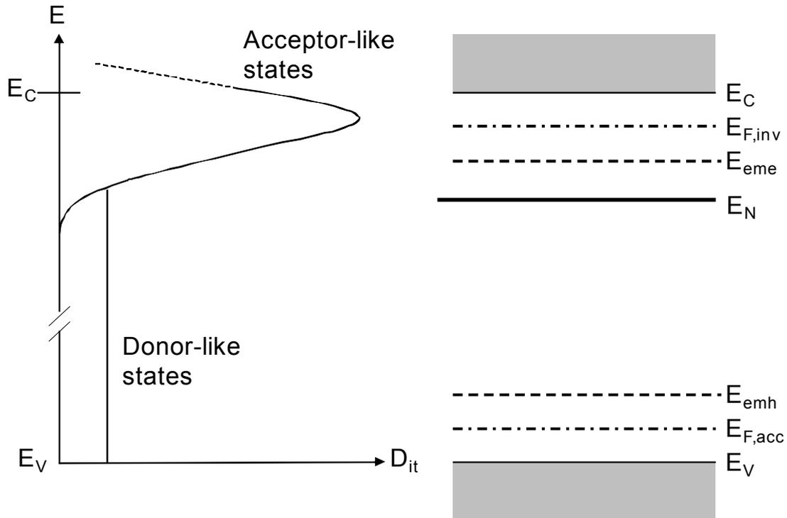
Fig. 5.8. Schematic illustration of the distribution of interface state density and band diagram.
