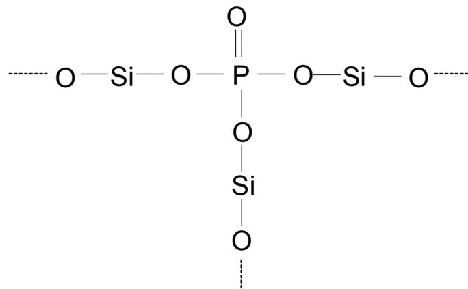
Fig. 4.10. Structure of P-doped  $\text{SiO}_2$  formed by  $\text{POCl}_3$  annealing of 4H-SiC.
