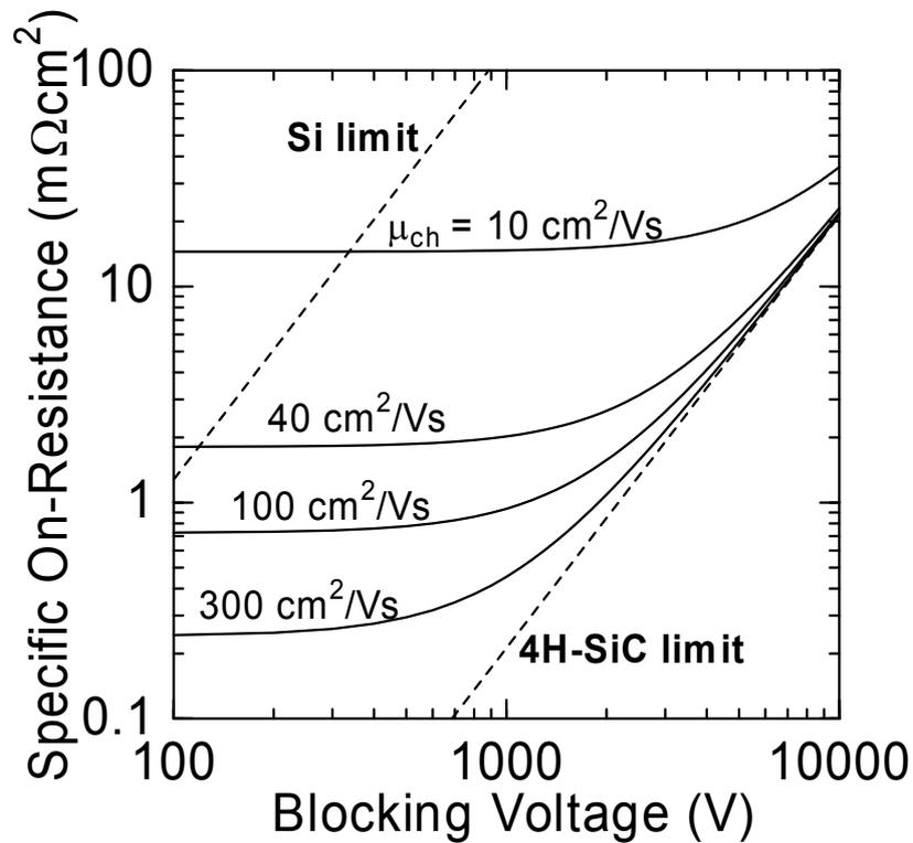
Fig. 1.6. Limit of specific on-resistance in Si and 4H-SiC power DMOSFETs as a function of blocking voltage and channel mobility, assuming that  $L = 1 \mu\text{m}$ ,  $P = 15 \mu\text{m}$ ,  $\mathcal{E}_{\text{ox}} = 3 \text{ MV/cm}$ .
