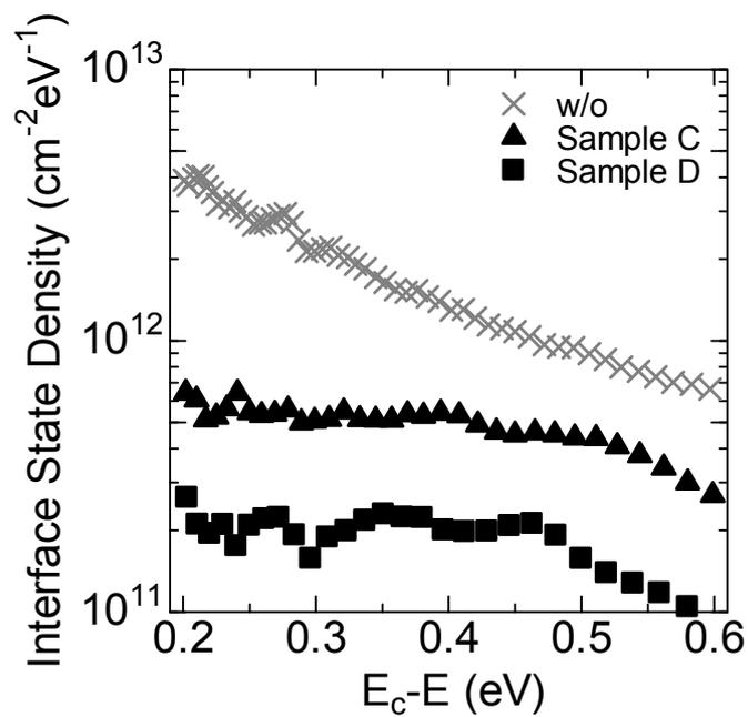
Fig. 6.12. Distribution of  $D_{it}$  for samples C and D estimated by the hi-lo  $C-V$  method.
