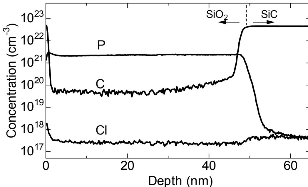
Fig. 3.8. P, C, and Cl atom profiles in the oxide and near the SiO<sub>2</sub>/4H-SiC interface annealed with POCl<sub>3</sub> at 1000 °C determined by SIMS measurements.
