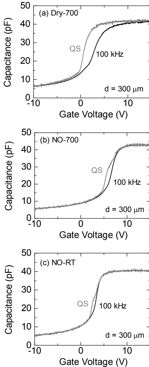
Fig. 6.4. high-frequency (100 kHz) and quasi-static  $C-V$  curves of C-face 4H-SiC MOS capacitors fabricated by the (a) Dry-700, (b) NO-700 and (c) NO-RT processes.
