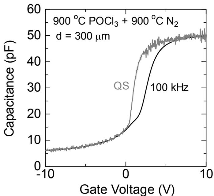
(a)  $\text{POCl}_3$  annealing at  $900\text{ }^\circ\text{C}$  followed by  $\text{N}_2$  annealing at  $900\text{ }^\circ\text{C}$
