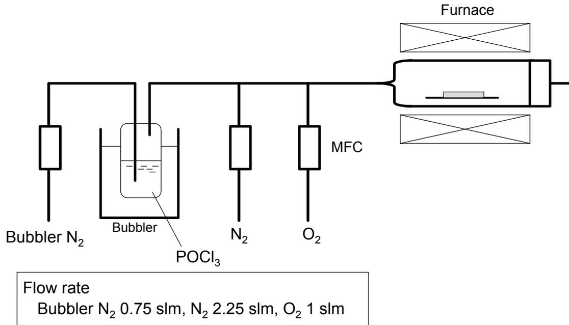
Fig. 3.1. POCl<sub>3</sub> annealing system used in this study.
