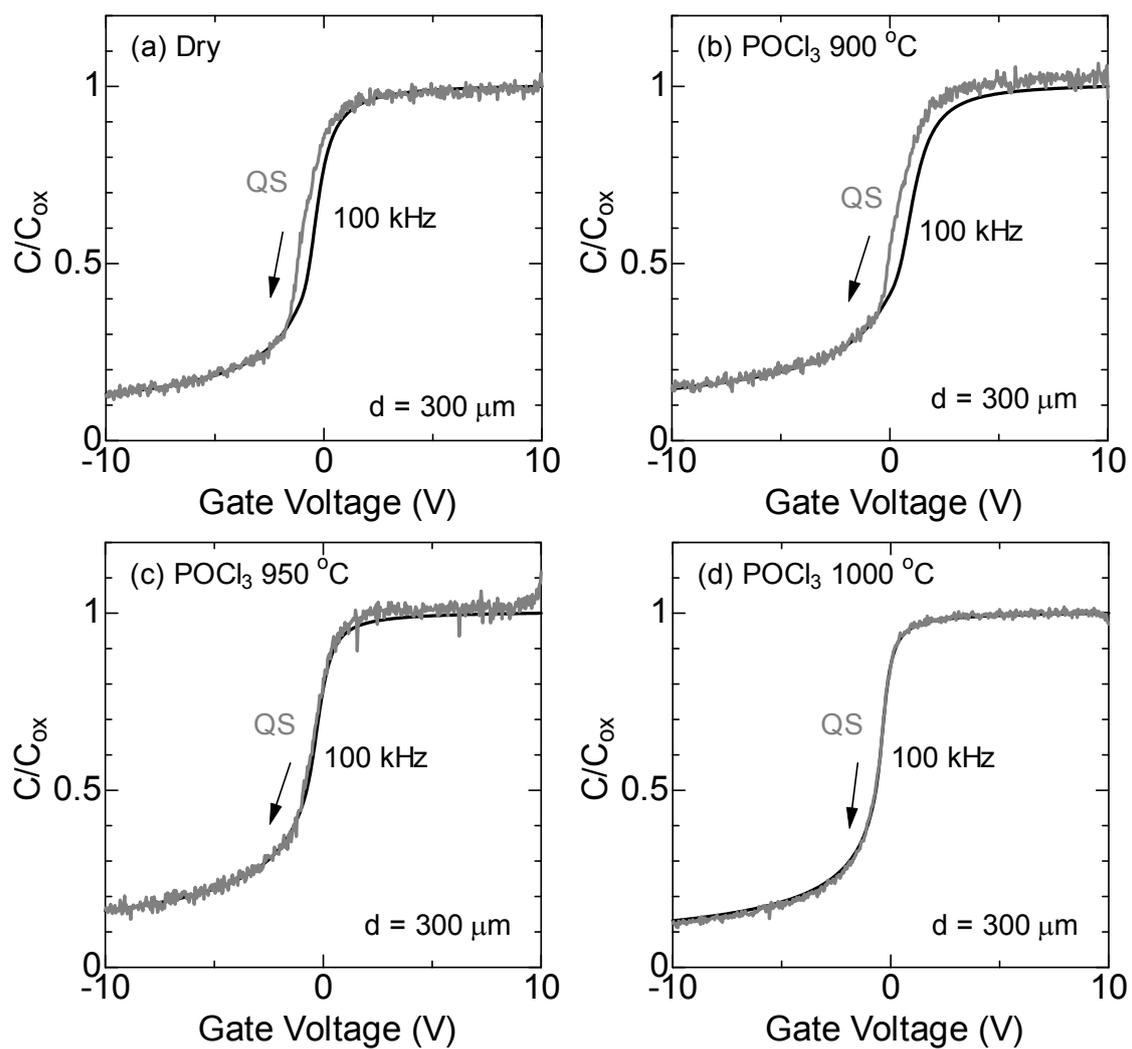
Fig. 3.3. High-frequency (100 kHz) and quasistatic (QS)  $C$ - $V$  curves for the dry and  $\text{POCl}_3$ -annealed oxides: (a) dry, (b)  $\text{POCl}_3$  annealing at 900 °C, (c)  $\text{POCl}_3$  annealing at 950 °C, and (d)  $\text{POCl}_3$  annealing at 1000 °C.
