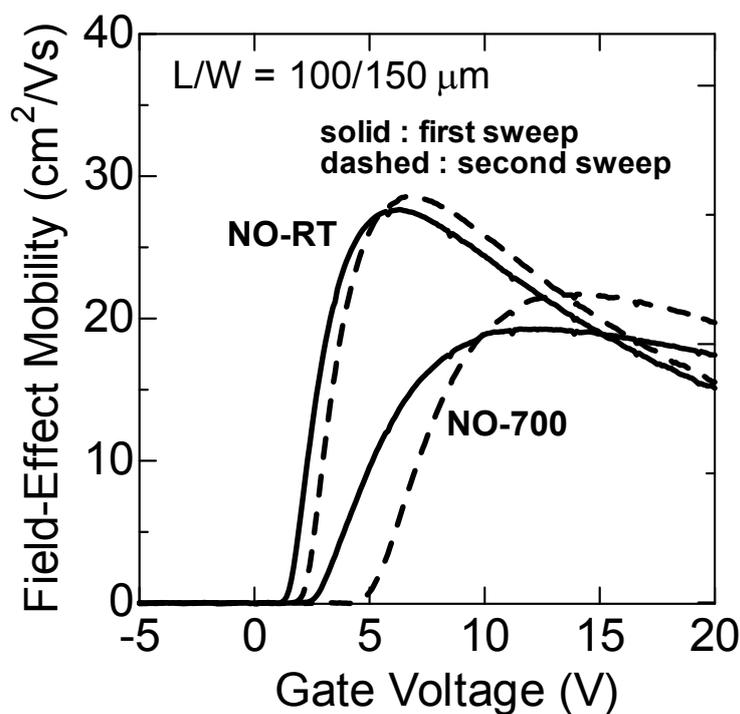
Fig. 6.7. Field-effect mobility of C-face 4H-SiC MOSFETs fabricated by the NO-700 and NO-RT processes.
