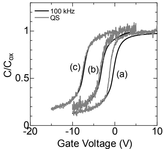
Fig. 2.7. High-frequency and quasistatic  $C-V$  curves of N-implanted MOS capacitors with implantation dose of (a)  $1.0 \times 10^{12}$ , (b)  $5.0 \times 10^{12}$ , and (c)  $1.0 \times 10^{13} \text{ cm}^{-2}$ .
