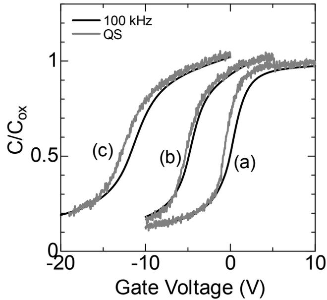
Fig. 2.6. High-frequency and quasistatic  $C-V$  curves of P-implanted MOS capacitors with implantation dose of (a)  $1.0 \times 10^{12}$ , (b)  $5.0 \times 10^{12}$ , and (c)  $1.0 \times 10^{13} \text{ cm}^{-2}$ .
