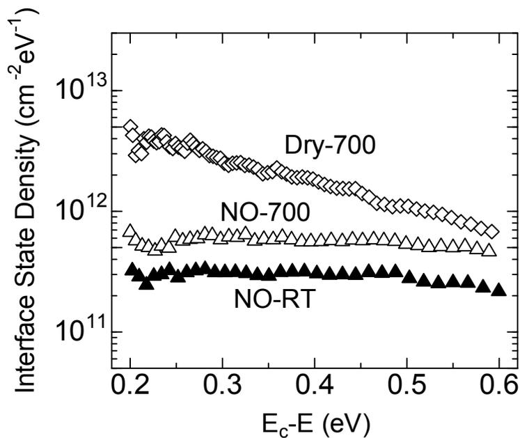
Fig. 6.5. Distribution of interface state density near the conduction band edge of C-face 4H-SiC MOS capacitors fabricated by the Dry-700, NO-700 and NO-RT processes.
