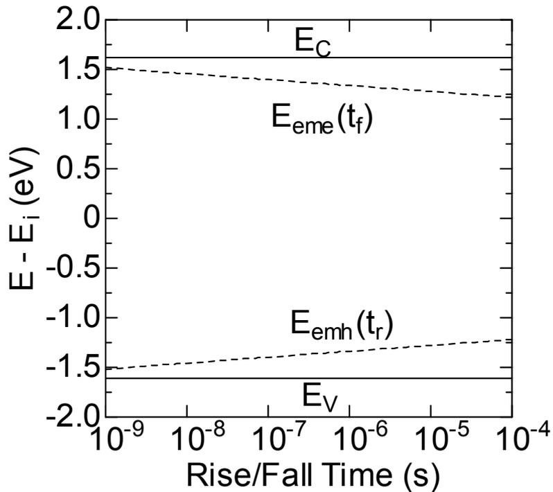
Fig. 5.11. Scannable energy interval for 4H-SiC MOSFETs as a function of pulse rise and fall times. Conduction and valence band edge are shown by solid lines. Dashed lines represent the energy level reached at the end of hole and electron emission. The energy difference  $|E_{eme}(t_f) - E_{emh}(t_r)|$  corresponds to the scanning energy range  $\Delta E$ .
