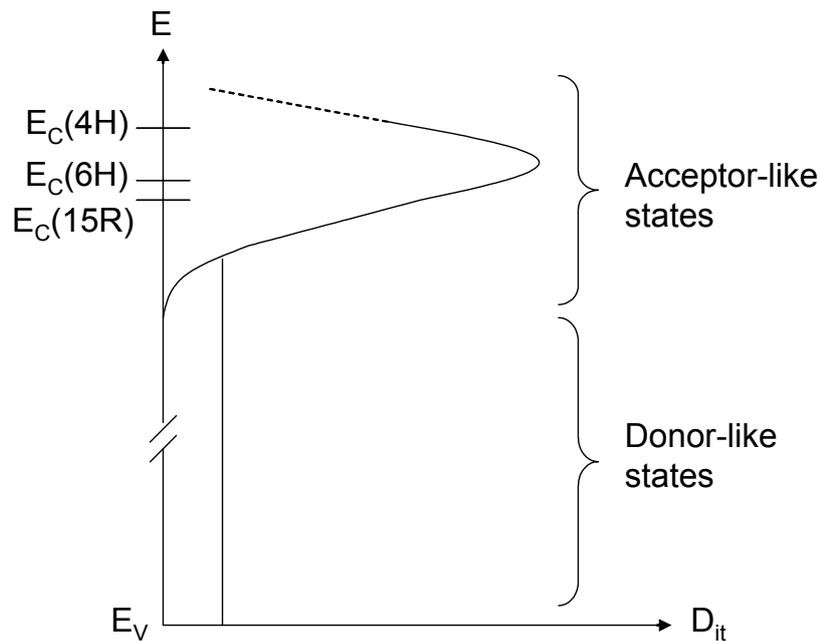
Fig. 1.8. Model for the distribution of interface states proposed by Schörner *et al.* [35].
