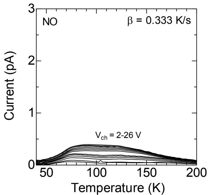
Fig. 4.6. Charging-voltage dependence of TDRC curves for the NO-annealed oxide.
