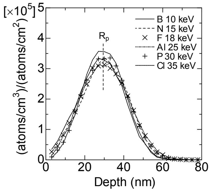
Fig. 2.1. Implantation profile for each element calculated with a SRIM code.
