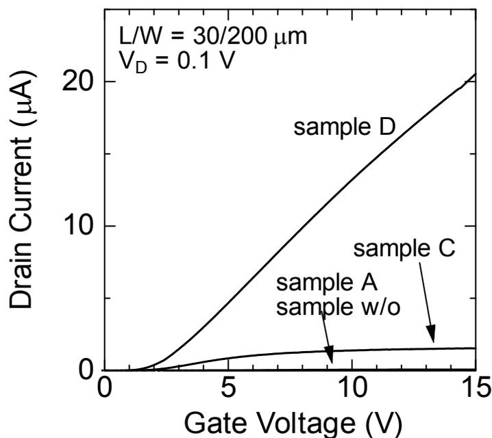
Fig. 6.14. Transfer characteristics of 4H-SiC MOSFETs fabricated on the C-face by  $\text{POCl}_3$  annealing followed by  $\text{N}_2$  annealing at various temperatures. The best result was obtained for the sample D which was fabricated by  $\text{POCl}_3$  annealing at  $900 \text{ }^\circ\text{C}$  followed by  $\text{N}_2$  annealing at  $1000 \text{ }^\circ\text{C}$ . The current was very small for samples A and w/o.
