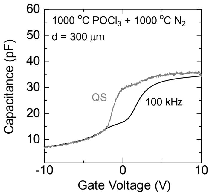
(b)  $\text{POCl}_3$  annealing at  $1000\text{ }^\circ\text{C}$  followed by  $\text{N}_2$  annealing at  $1000\text{ }^\circ\text{C}$
