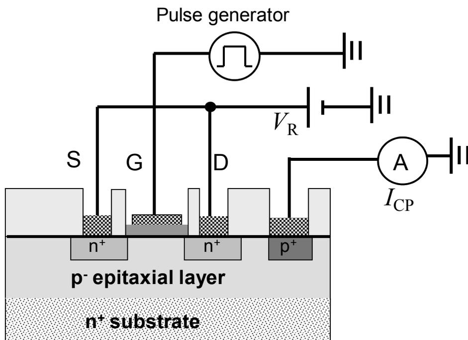
Fig. 5.1. Basic experimental setup for charge pumping measurements.
