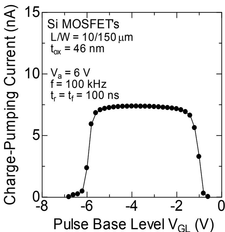
Fig. 5.5. Base-sweep charge-pumping curves for n-channel Si MOSFETs with a gate length  $L = 10 \mu\text{m}$  and gate width  $W = 150 \mu\text{m}$ . Pulse amplitude  $V_a = 6$  V, pulse frequency  $f = 100$  kHz, and pulse rise and fall times of  $t_r = t_f = 100$  ns.
