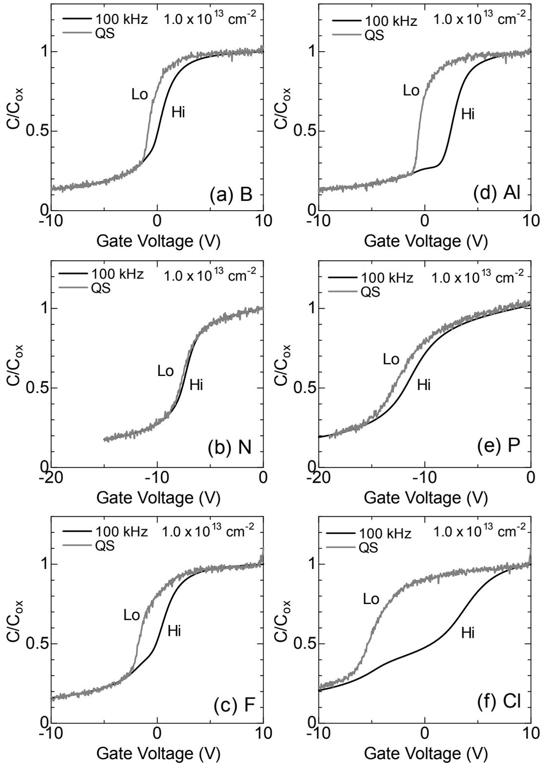
Fig. 2.5. High-frequency and quasistatic  $C-V$  curves for (a) B-, (b) N-, (c) F-, (d) Al-, (e) P-, and (f) Cl-implanted samples. The implantation dose is  $1.0 \times 10^{13} \text{ cm}^{-2}$ .
