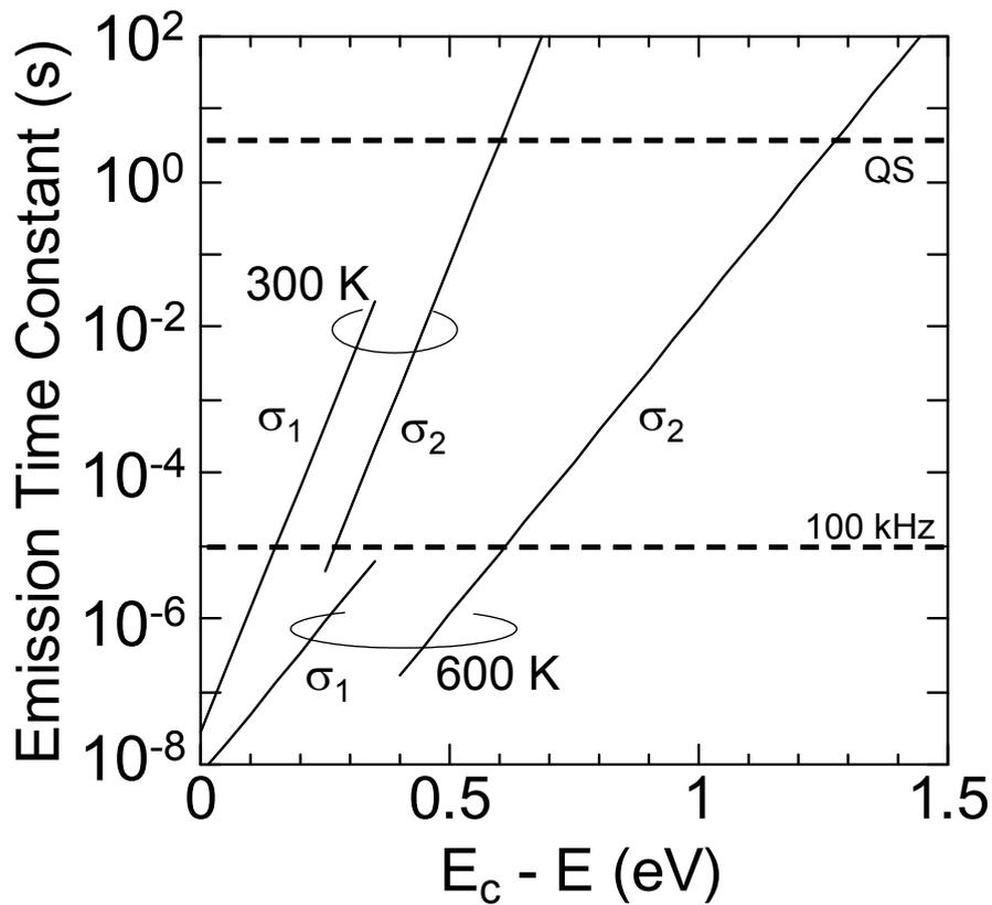
Fig. 2.4. Emission time constant as a function of trap energy level ( $E$ ) from the conduction band edge ( $E_c$ ). The capture cross section was assumed to be independent of temperature and  $1 \times 10^{-19} \text{ cm}^2$  for shallower states ( $\sigma_1$ ) and  $1 \times 10^{-17} \text{ cm}^2$  for deeper states ( $\sigma_2$ ) [22].
