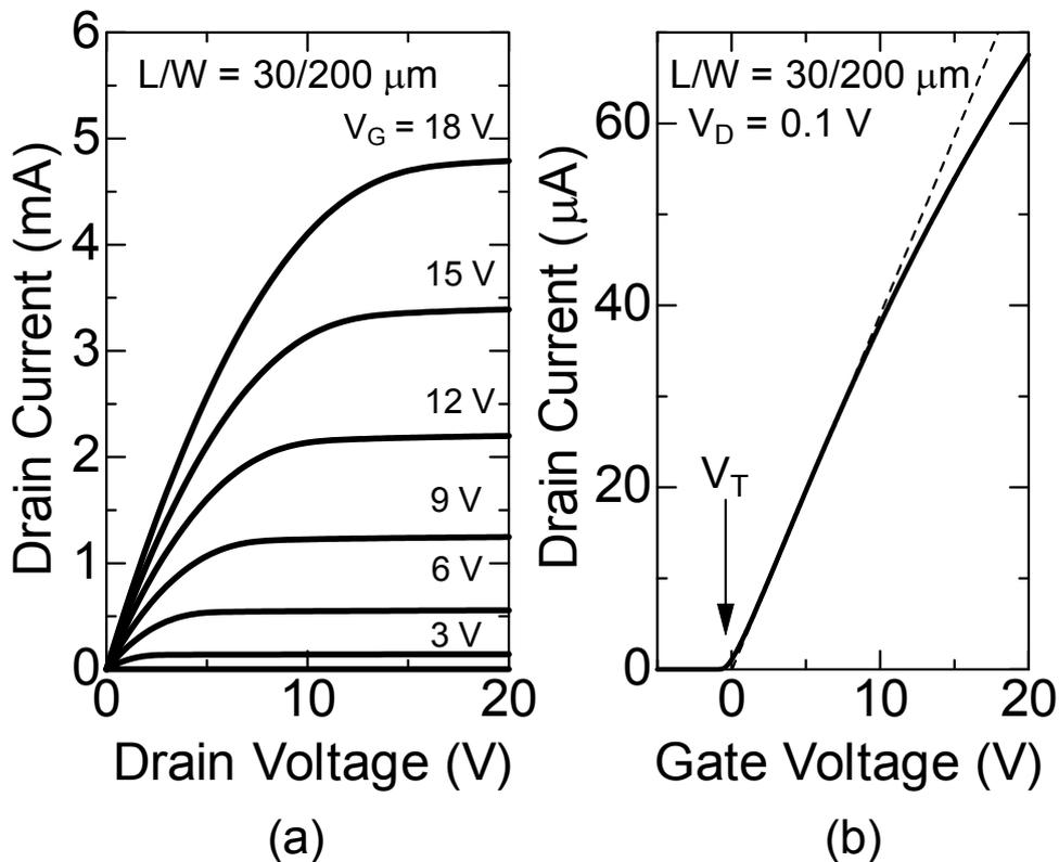
Fig. 3.5. (a) Output and (b) transfer characteristics of 4H-SiC MOSFETs fabricated on the Si-face by  $\text{POCl}_3$  annealing at 1000 °C.
