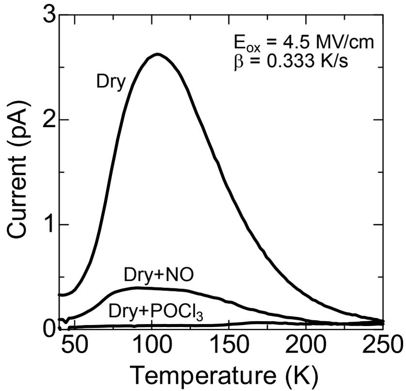
Fig. 4.3. TDR spectra for dry, NO-annealed, and POCl<sub>3</sub>-annealed oxides. Electric field across the oxide during charging was approximately 4.5 MV/cm. Heating rate ( $\beta$ ) is 0.333 K/s. Discharging voltage ( $V_{\text{dis}}$ ) is  $-5 \text{ V}$ .
