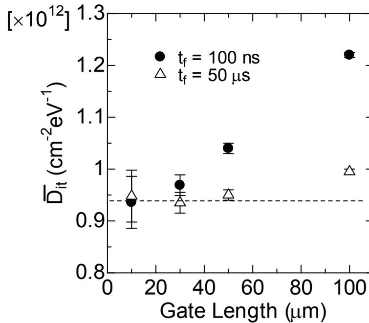
Fig. 5.13. Estimated mean interface state density as a function of gate length.
