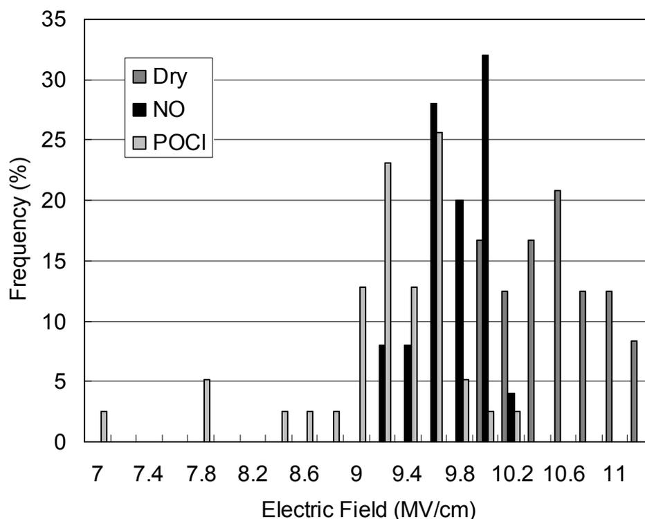
Fig. 3.10. Distributions of field-to-breakdown ( $\mathcal{E}_{DB}$ ) of dry, NO-annealed, and POCl<sub>3</sub>-annealed oxides obtained from TZDB measurements at room temperature.
