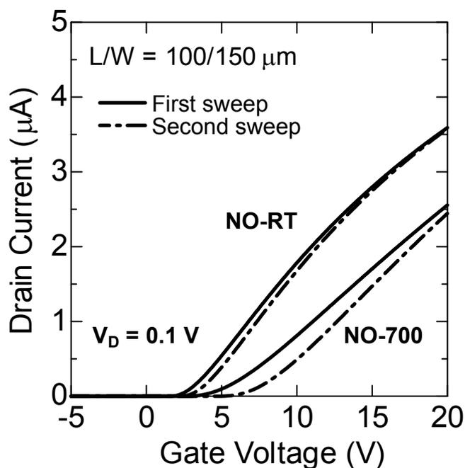
Fig. 6.6.  $I_D$ - $V_G$  characteristics at  $V_D = 0.1$  V for C-face 4H-SiC MOSFETs fabricated by the NO-700 and NO-RT processes. The solid line shows the first sweep and the dashed line shows the second sweep.
