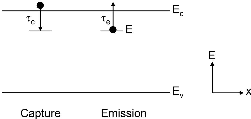
Fig. 2.2. Schematic illustration of the capture and emission process of an electron.
