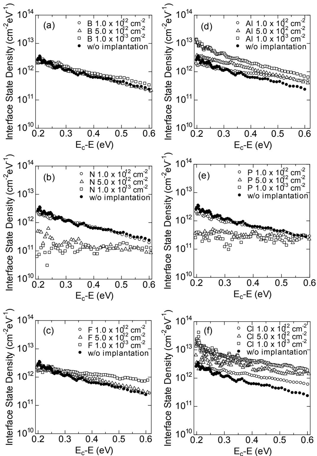
Fig. 2.8. Interface state density near the conduction band edge for (a) B-, (b) N-, (c) F-, (d) Al-, (e) P-, and (f) Cl-implanted samples.
