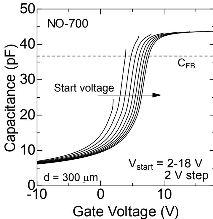
Fig. 6.2. Start voltage dependence of high-frequency  $C$ - $V$  curves for a C-face 4H-SiC MOS capacitor fabricated by the NO-700 process. Diameter of the circular gate electrode is  $300 \mu\text{m}$ . The gate voltage was swept from accumulation to depletion. The start voltage was increased from 2 to 18 V with a 2-V step.
