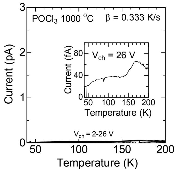
Fig. 4.7. Charging-voltage dependence of TDRC curves for the  $\text{POCl}_3$ -annealed oxide.
