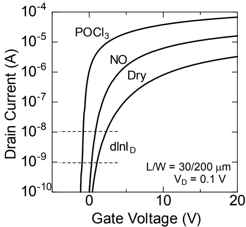
Fig.3.7. Subthreshold characteristics of 4H-SiC MOSFETs fabricated on the Si-face by dry oxidation, NO annealing, and the POCl<sub>3</sub> annealing at 1000 °C.
