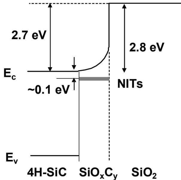
Fig. 4.4. Rudenko's interface model [2]. Near-interface traps (NITs) are assumed to be intrinsic interfacial defects energetically located near the conduction band edge of 4H-SiC and spatially distributed from the interface into the oxycarbide transition region.
