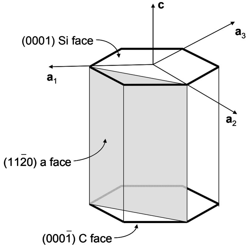
Fig. 1.3. Hexagonal unit cell and important crystal orientations.
