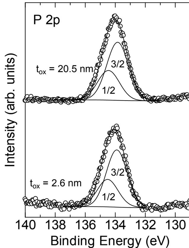
Fig. 4.9. P2p XPS spectrum of the  $\text{POCl}_3$ -annealed oxide. The oxide thickness was about 20.5 and 2.6 nm. The take-off angle was  $90^\circ$ .
