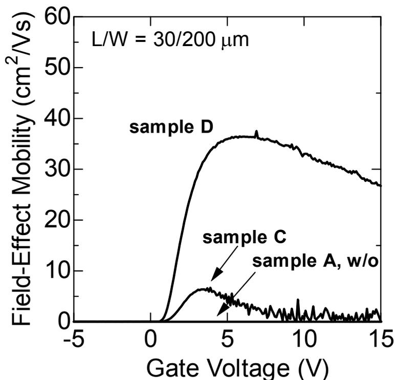
Fig. 6.15. Field-effect mobility of 4H-SiC MOSFETs fabricated on the C-face by  $\text{POCl}_3$  annealing followed by  $\text{N}_2$  annealing at various temperatures. The best result was obtained for the sample D which was fabricated by  $\text{POCl}_3$  annealing at  $900^\circ\text{C}$  followed by  $\text{N}_2$  annealing at  $1000^\circ\text{C}$ . The mobility was very small for samples A and w/o.
