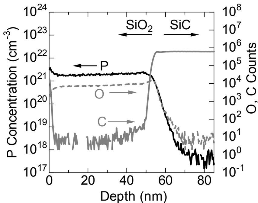
Fig. 6.13. SIMS profile for the sample D which was fabricated by  $\text{POCl}_3$  annealing at  $900^\circ\text{C}$  followed by  $\text{N}_2$  annealing at  $1000^\circ\text{C}$ .
