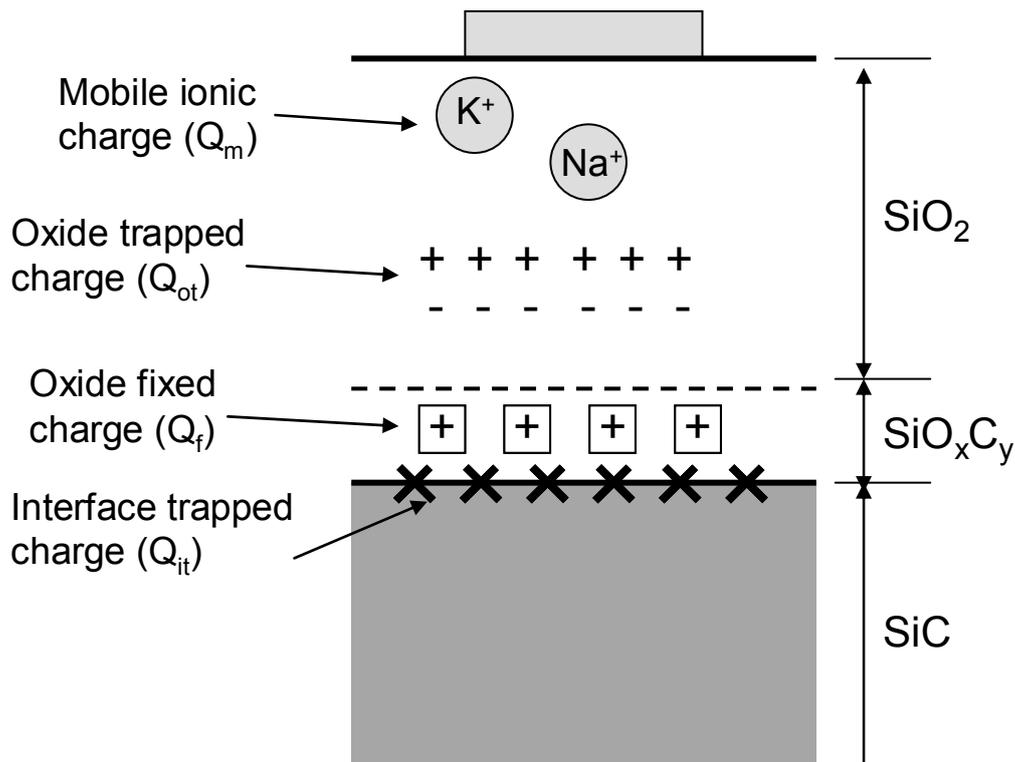
Fig. 1.7. The basic classifications of the charges at the interface and in the oxide [7].
