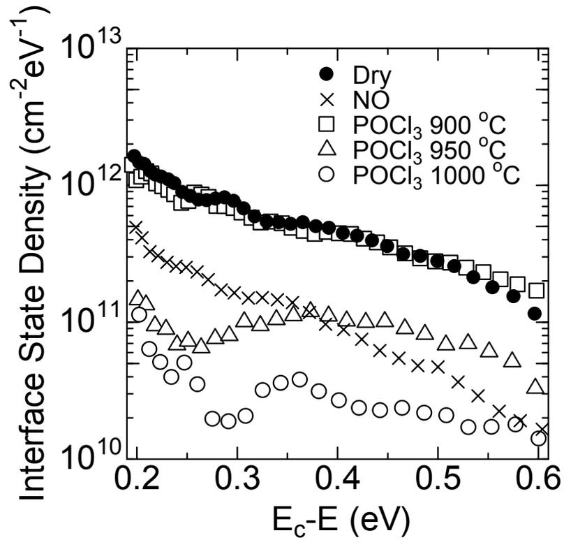
Fig. 3.4. Energy distribution of interface state density near the conduction band edge obtained from the hi-lo  $C-V$  method for P-doped oxides annealed at 900 °C, 950 °C, and 1000 °C. The results of dry and NO-annealed oxides are also shown.
