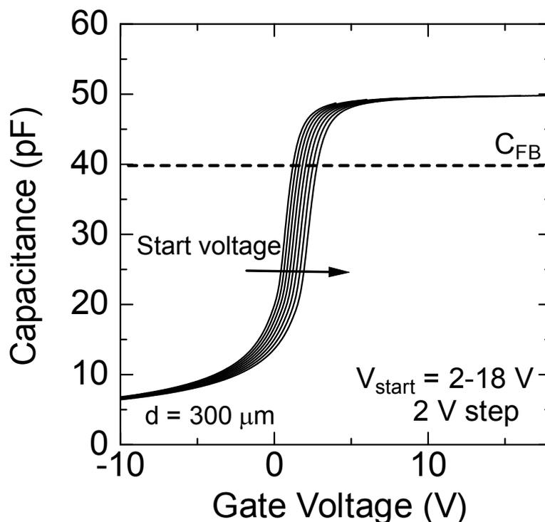
Fig. 6.16. Start voltage dependence of high-frequency  $C$ - $V$  curves for a C-face 4H-SiC MOS capacitor fabricated by  $\text{POCl}_3$  annealing at  $900\text{ }^\circ\text{C}$  followed by  $\text{N}_2$  annealing at  $1000\text{ }^\circ\text{C}$  (sample D). Diameter of the circular gate electrode is  $300\text{ }\mu\text{m}$ . The gate voltage was swept from accumulation to depletion. The start voltage was increased from 2 to 18 V with a 2-V step.
