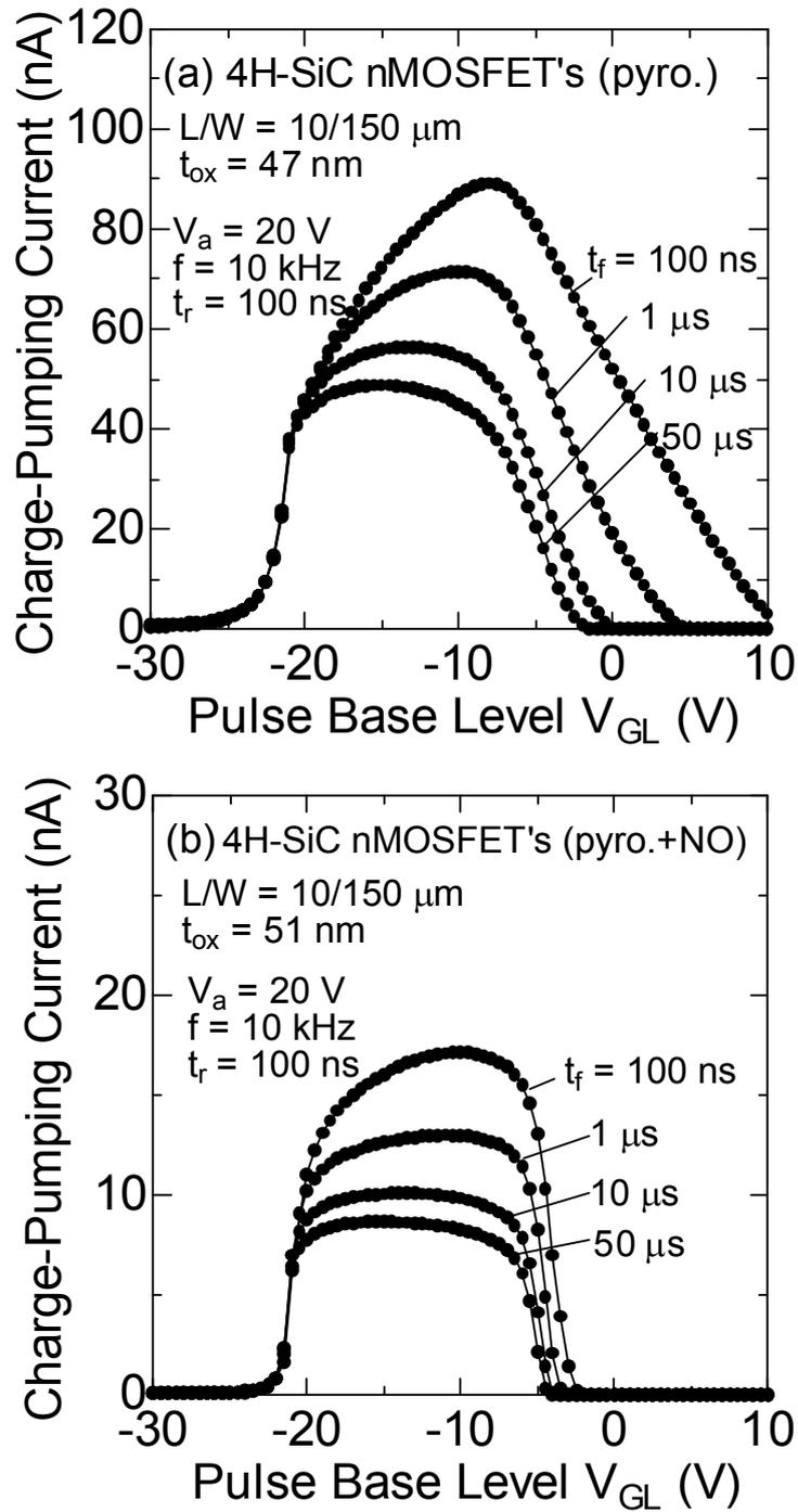
Fig. 5.6. Pulse-fall-time dependence of base-voltage sweep charge-pumping curves for (a) unannealed n-channel 4H-SiC MOSFETs and (b) NO-annealed 4H-SiC n-channel MOSFETs with gate length  $L = 10 \mu\text{m}$  and gate width  $W = 150 \mu\text{m}$ . Pulse amplitude  $V_a = 20 \text{ V}$ , pulse frequency  $f = 10 \text{ kHz}$ , and pulse rise time  $t_r = 100 \text{ ns}$ .
