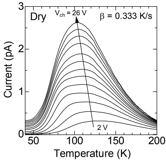
Fig. 4.5. Charging-voltage dependence of TDRC curves for the dry oxide.
