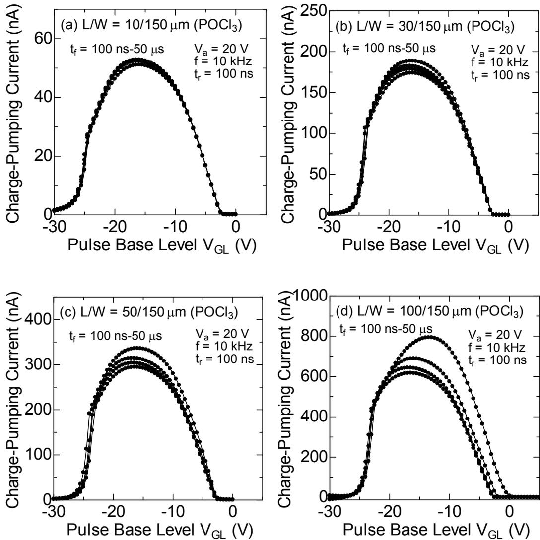
Fig. 5.12. Pulse-fall-time dependence of base-voltage sweep charge-pumping curves for  $\text{POCl}_3$ -annealed 4H-SiC MOSFETs with gate length  $L = 10, 30, 50, 100 \mu\text{m}$  and gate width  $W = 150 \mu\text{m}$ . Pulse amplitude  $V_a = 20 \text{ V}$ , pulse frequency  $f = 10 \text{ kHz}$ , and pulse rise time  $t_r = 100 \text{ ns}$ .
