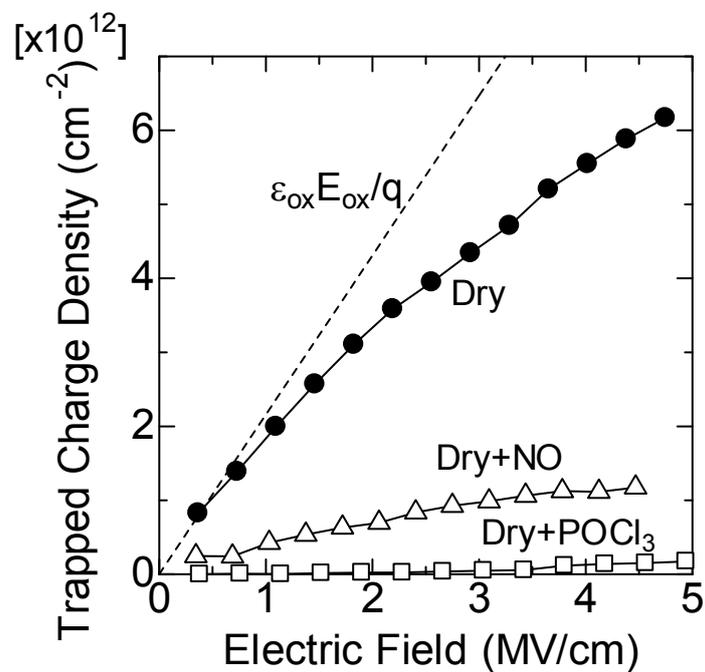
Fig. 4.8. Density of trapped electrons in interface traps as a function of electric field across the oxide during charging. Dashed line denotes the total accumulated charge at the  $\text{SiO}_2/4\text{H-SiC}$  interface during charging.
