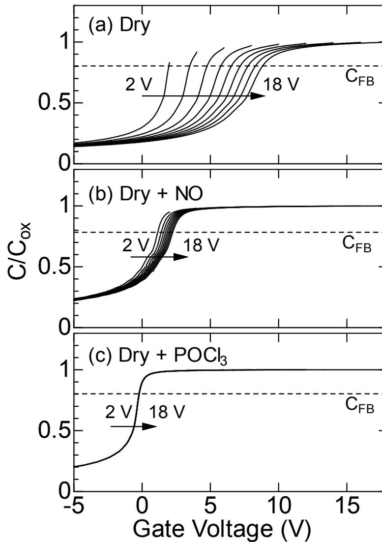
Fig. 4.1. Start voltage dependence of high-frequency (100 kHz)  $C-V$  curves measured at 80 K for (a) dry, (b) NO-annealed, and (c)  $\text{POCl}_3$ -annealed oxides. The gate voltage was swept from accumulation to depletion (positive to negative). Start voltage was increased from 2 to 18 V in a 2-V step. Dashed lines denote the flatband capacitance ( $C_{\text{FB}}$ ).
