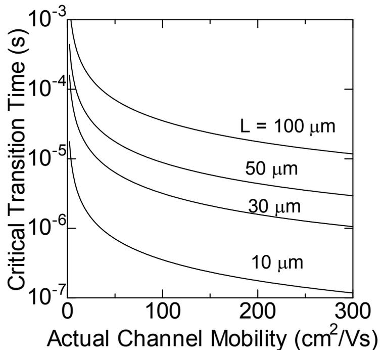
Fig. 5.10. Calculated critical transition time as a function of *actual* channel mobility for gate lengths of 10, 30, 50, and 100  $\mu\text{m}$ . The critical transition time is defined as the time required to reduce the density of channel electrons from  $10^{13}$  to  $10^9 \text{ cm}^{-2}$ .
