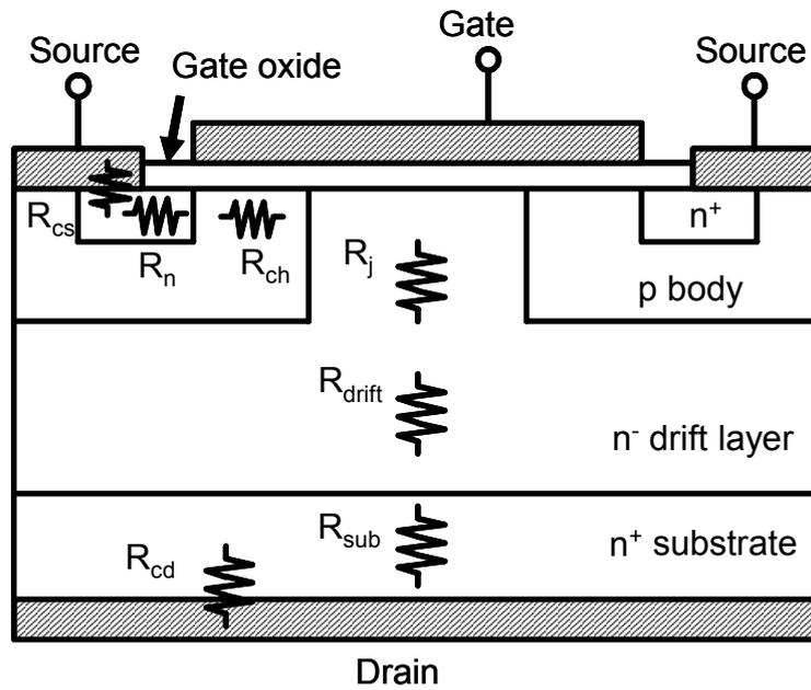
Fig. 1.4. Typical structure of a SiC DMOSFET and various contributions to the on-resistance.
