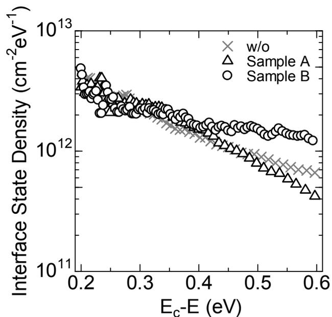
Fig. 6.10. Distribution of  $D_{it}$  for samples A and B estimated by the hi-lo  $C-V$  method.
