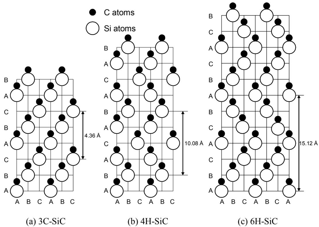
Fig. 1.2. Stacking orders of (a) 3C-, (b) 4H-, and (c) 6H-SiC. Open and closed circles indicate Si and C atoms, respectively.
