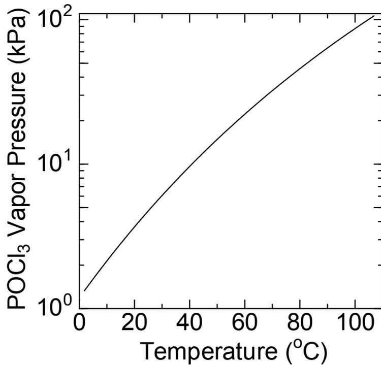
Fig. 3.2. Vapor pressure of POCl<sub>3</sub>.
