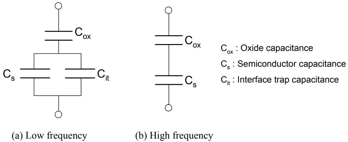
Fig. 2.3. (a) Low-frequency and (b) high-frequency equivalent circuits of the MOS capacitor.
