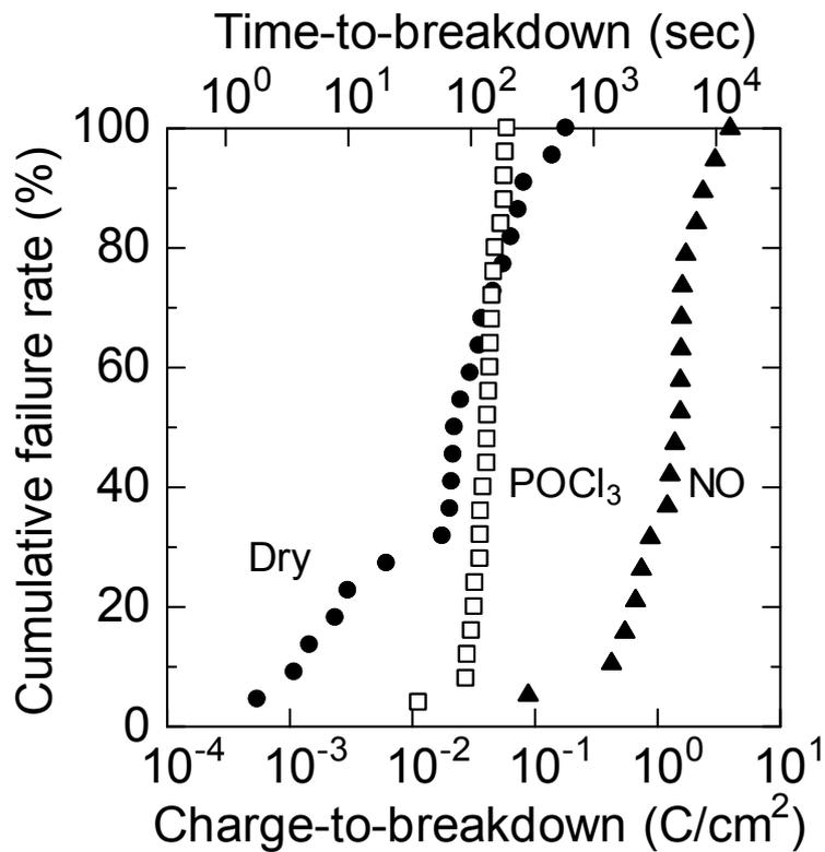
Fig. 3.11. The distribution of cumulative failure rate for dry, NO-annealed, and POCl<sub>3</sub>-annealed MOS capacitors.
