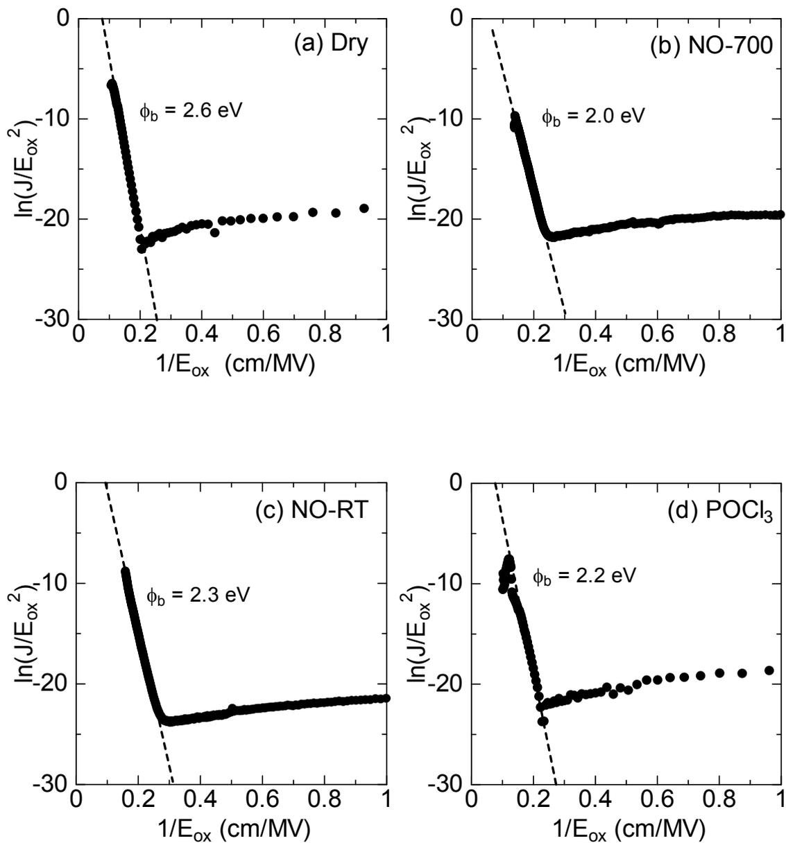
Fig. 6.18. FN plots of (a) dry, (b) NO-700, (c) NO-RT, and (d) POCl<sub>3</sub>-analed (sample D) MOS capacitors on C-face 4H-SiC.
