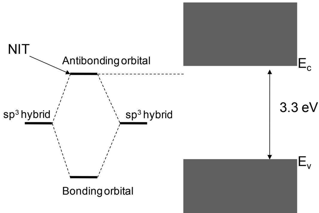
Fig. 4.11. Schematic of Si–Si bonding-antibonding states. Si–Si bonds have bonding-antibonding energy splittings depending on the bond length and could give rise to localized states near the band edges [17].
