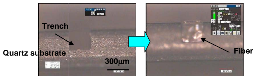
Figure 3.13: Cross-sectional microscope images of the fiber embedded into the trench formed in a quartz substrate.
