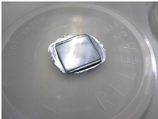
Figure 3.15 Photograph of 15 \mu\text{m} c-Si foil adhered on glass superstrate after separation
