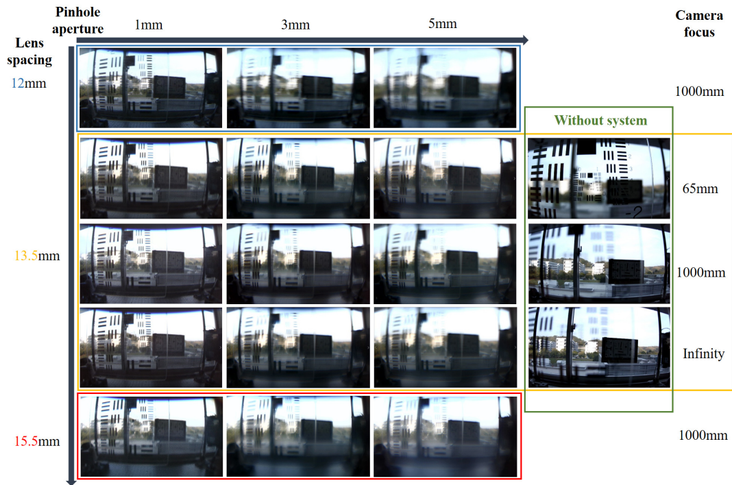
Figure 3.6: See-through views tested with various pinhole apertures, lens spacings, and the camera focuses.
