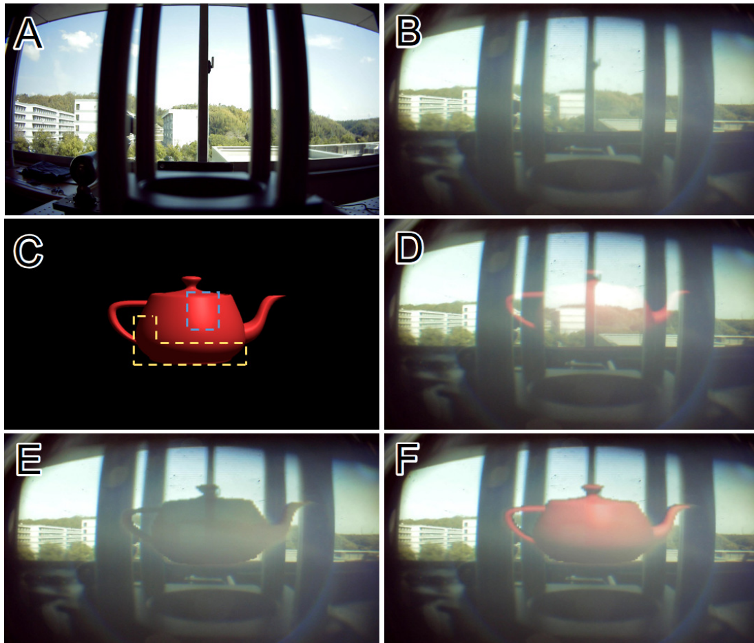
Figure 4.12: Hard-edge occlusion is demonstrated by the prototype of the R-PPM system with the recorded FOV of H83.5^{\circ} \times V53.1^{\circ} .
