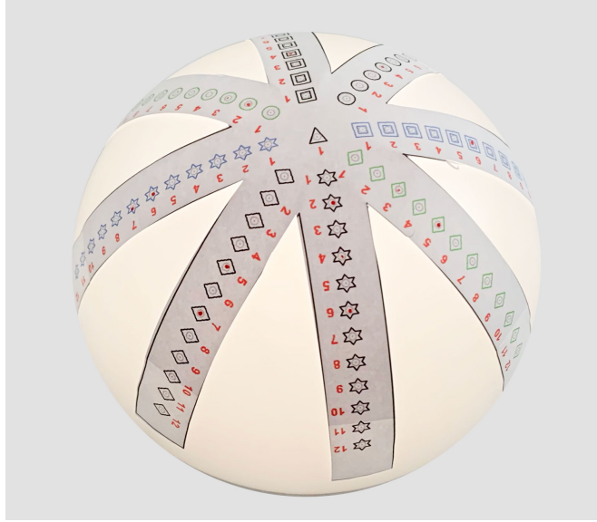
Figure 19: A half sphere with targets. Each target was marked by an empty symbol 3 mm, inner circle 1.2 mm, and an inner dot of 0.34 mm. The targets were numbered from the top (no. 1) towards the edge (no. 12).
