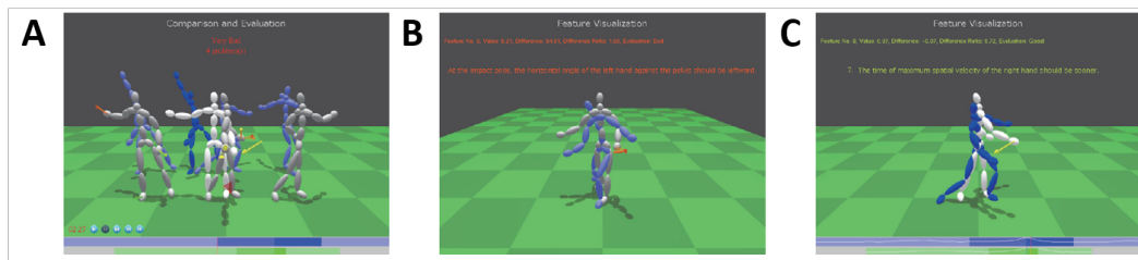
Figure 4.13: Self-training system for tennis shots (adapted from [14]), (A) comparison and evaluation mode for trainee and target motions, (B) isolated key poses indicated by gray and light blue, (C) isolated trainee pose in white and target pose in blue.
