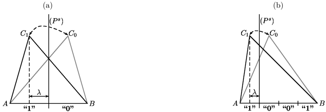
Figure 4.3: Cayre et al. [12]. One bit is encoded by moving the vertex C to C_0 or C_1 position such that its projection on the edge AB is in a “0” or “1” region. (a) two regions, more robust but bigger deformation required. (b) four regions, less robust but smaller deformation required.
