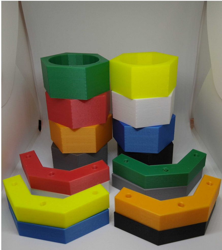
Figure 6.16: Objects used for color robustness evaluation Each object was printed with a PLA filament, 0.2mm layer thickness, and signal amplitude \alpha = 40\% .
