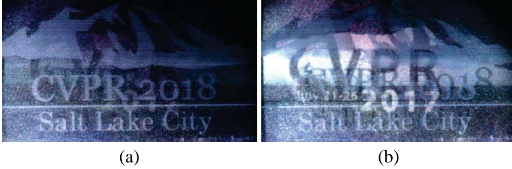
Figure 5.11: Reconstruction of reflectance maps in two layers. The target object consists of two OHP sheets on which CVPR logos are printed.
