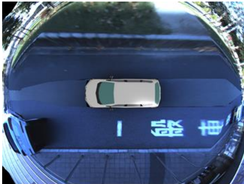
(b) A virtual viewpoint image with improved resolution by the method proposed in Chapter 4 ( N_t=N_p=6 ).
