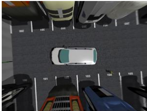
(a) An image generated using left and right camera images in overlapping area.
