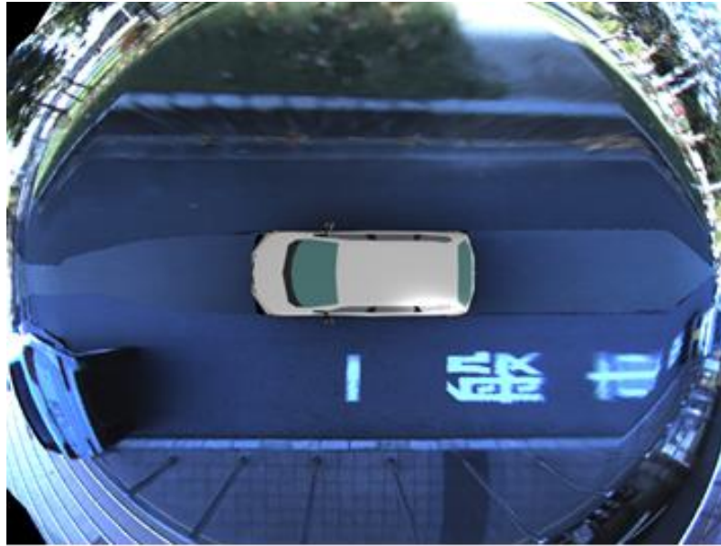
(a) A virtual viewpoint image generated by the method proposed in Chapter 3. (Composite projection, a half-pipe shape model)
