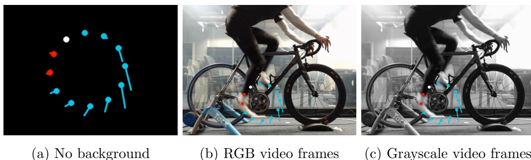
Figure 3.7: The vector-based data visualization for representing pedaling forces.
