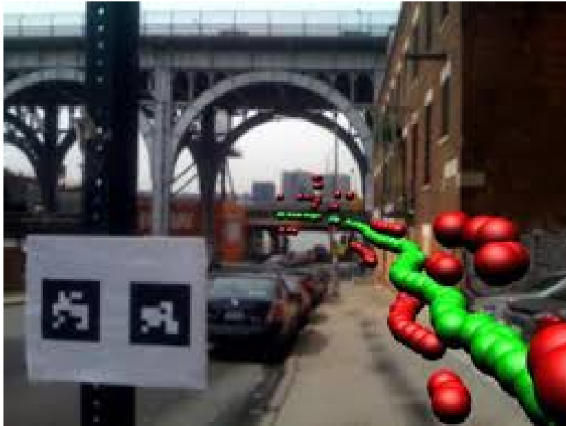
Figure 3.4: White's situated visualization. Spheres represent carbon monoxide data captured at the exact location to emphasize the effects of environment [190].
