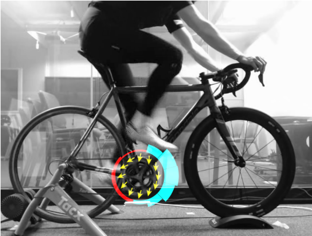
Figure 3.9: Grayscale video frames are combined with independent visualizations of force direction and torque generation. Blue color represent positive contribution to rotation whereas red represents vice versa.
