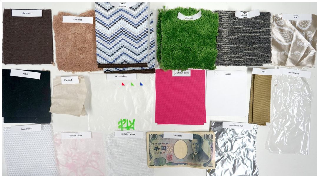
Figure 46. Single and multiple layers of the 18 materials were distinguished for a total of 36 cases. The case with two layers of cushion (top row, 3rd from the left) was excluded due to the high thickness.
