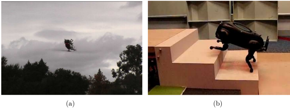
Figure 2.4.: Examples of reinforcement learning in robotics: a) Helicopter learning controller for inverted flight [57], b) Four legged little dog robot learning controller for climbing stairs [59].
