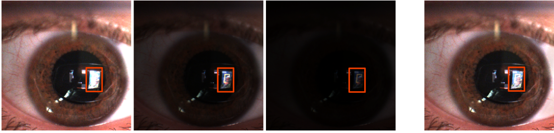
Figure 38. Combining 3 frames obtained from the HDR camera (left) with Exposure Fusion to reveal the full dynamic of the corneal image at night time (right).
